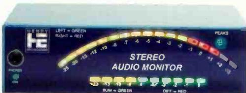
indicate phase error or a polarity reversal in the audio chain. The meter accepts either an AES/EBU digital input or analog inputs. It accurately indicates system levels over a range of -25 to +3 VU. A headphone jack is provided for aural monitoring.
