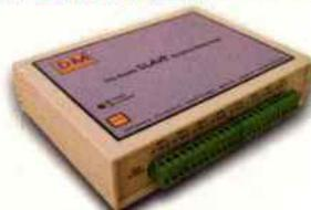
The Studio SLAVE Auxiliary Relay Pack from DM Engineering is an economical solution for studio control functions at about one-half the price of competing products, featuring 8 form C contacts for switching functions, ranging from low level audio up to 2 amps of AC or DC. Momentary, latching, positive DC and logic low input control. The Studio SLAVE also features steady state and flashing Solid State Relay driver voltages, variable relay release delay and more.
