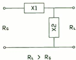
is a virtual quantity; however, it is usually adjusted in order to meet a desired Q value, and by extension, bandwidth across the network. Note that in the Pi network this virtual impedance will be lower than either the generator or load impedance because the shunt legs of the two L networks are opposite each other. The reverse is true for the T network.
