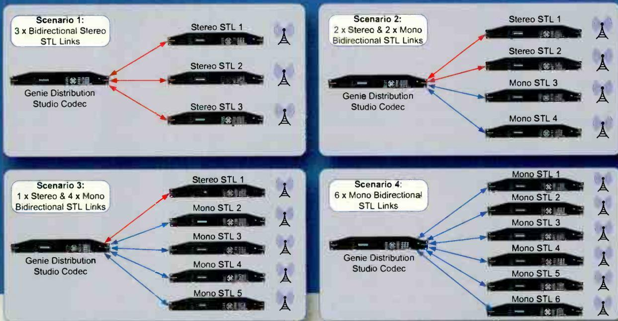
Connect 3 independent stereo streams or, 2 stereo + 2 mono, or 1 stereo + 4 mono, or 6 mono streams
