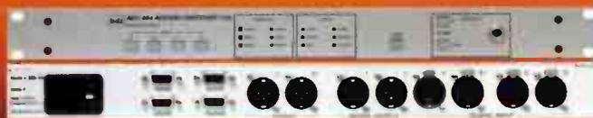
**AES-404** 4 Input Digital Audio Switcher—Provides two AES3 outputs and analog L/R +4 dBm balanced output. A great general purpose digital switcher where more than two inputs need to be accommodated. Serial and parallel remote control and front panel headphone output.
