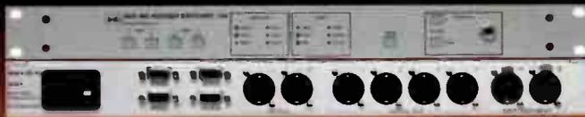
**AES-402** 2 Input Digital Audio Switcher— Provides four AES3 output DA and analog L/R +4 dBm balanced output. Automatic features include silence and error switching which are all user configurable. Now with serial and parallel remote control interface . Includes a front panel headphone output too!
