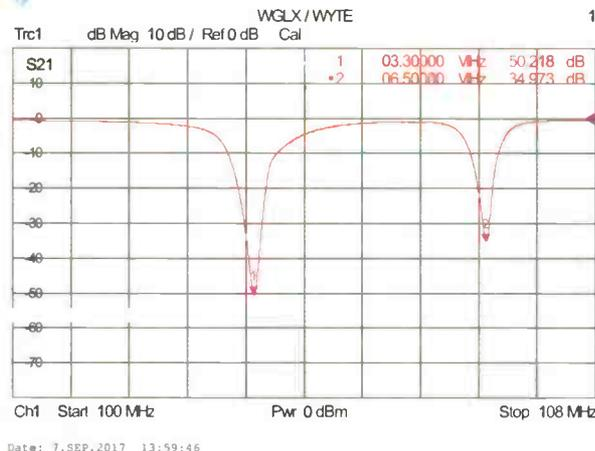
Network analyzer characterization of notch-filters to be used ahead of spectrum analyzer input. These filters reduce the amount of the fundamental signals getting in to the analyzer, which effectively increases the dynamic range of the measurement, allowing an easier “capture” of the actual IMD products, should they exist.
