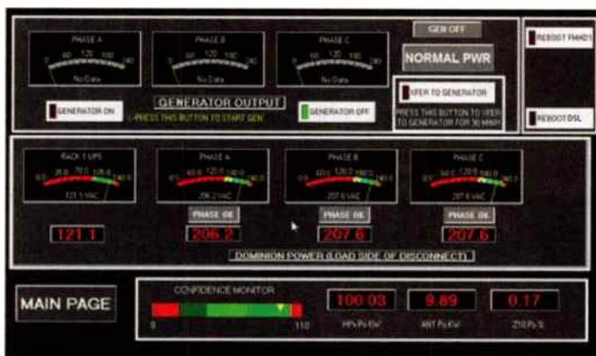
Metering for the "normal" side means that engineering can keep track of utility power as well as generator power.
