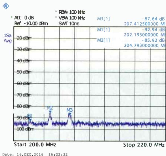
Spectrum analyzer results showing low-level IMD products.
