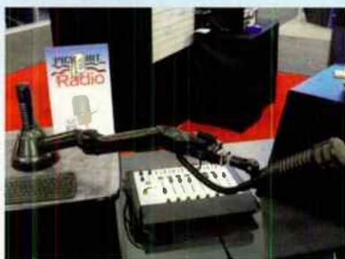
This patented system employs super quiet robotic motors and special facial recognition technology to determine the distance between the person's face and the tip of the microphone. Once the "RoboBoom" is engaged, it automatically positions the microphone at an optimal distance from the talent for best audio quality pickup.
