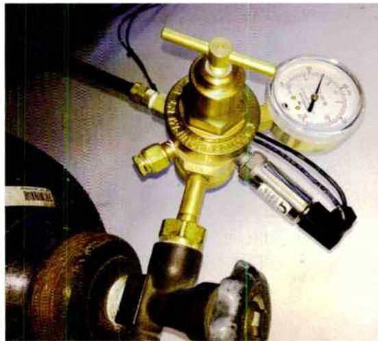
Figure 4: Omega tank pressure sensor
