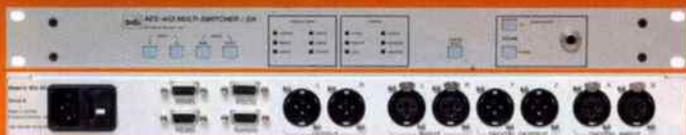
**AES-403** 2 Input Digital Audio Switcher— Accepts two AES3 inputs or one input can be configured to accept analog L/R + 4dBm input. Provides 2 - AES3 outputs and analog L/R + 4 dBm output. Use for EAS insertion or to insert analog into your digital path. Has AES-402 functionality including automatic features.
