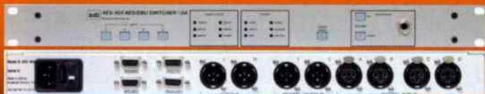
**AES-404** 4 Input Digital Audio Switcher— Provides two AES3 outputs and analog L/R +4 dBm balanced output. A great general purpose digital switcher where more than two inputs need to be accommodated. Serial and parallel remote control and front panel headphone output.
