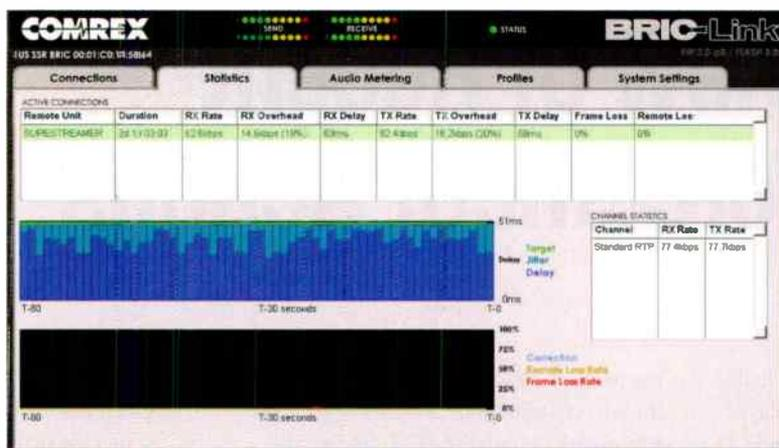
Fig. 2: Network Connection Statistic page of the BRIC Link at 1 Union Station.
