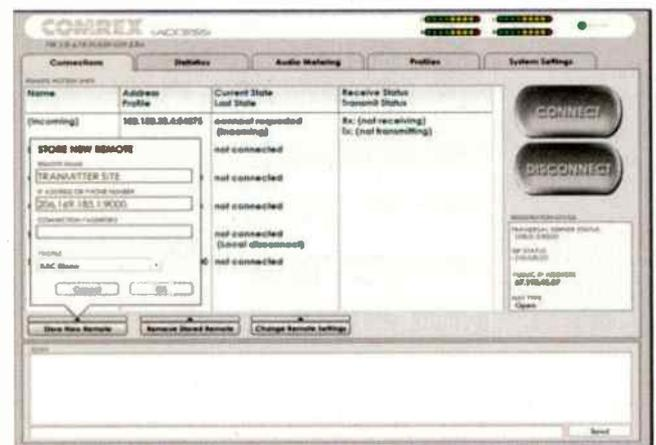
Fig. 3: Configuring a new remote connection
