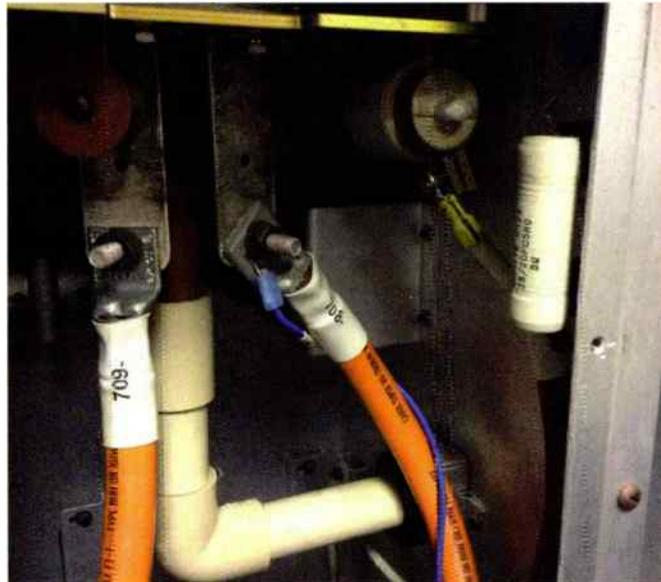
The final amplifier input section (below the tube socket) should be clean and inspected for loose or broken parts as part of the rebuild process.
