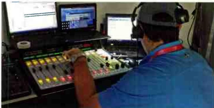
To learn how we made it all work using 4G iPhone 6s with Report-IT, Tieline Genie distribution, a 5W transmitter, and Wheatstone IP audio networking, audio processing and IP console...
