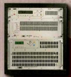
EM 2000 is a 2000W FM transmitter made up of the EM 25 DIG exciter (or EM 20/30 exciter) and the AM 2000 FM amplifier. AM 2000 includes eight 300W high-efficiency MOSFET technology amp ifying modules, fed by 2 independent switching power supplies, which are made to withstand the working conditions. The amplifying modules work independently thanks to a power combining structure that provides high isolation between them.
