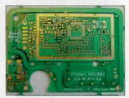
Board of FM receiver with internal antenna
