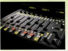
iQ: The iQ's package includes: a control surface, DSP-based mixing engine, audio I/O, machine-control logic, even a built-in Ethernet switch. Simply connect the control surface to the Core with a single cable, add audio inputs using CAT-5 cable, perform some fast Web-based configuration, and iQ is ready to broadcast. Simple networking lets users daisy-chain up to four iQ Cores without the
