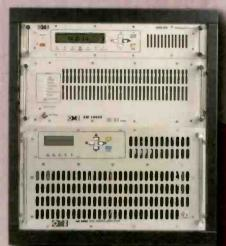
EM 2000 is a 2000W FM transmitter mode up of the EM 25 DIG exciter for EM 20/30 exciter) and the AM 2000 FM amplifier. AM 2000 includes eight 300W high-efficiency MOSFET technology amplifying modules, fed by 2 independent switching power supplies, which are mode to withstand the working conditions. The amplifying modules work independently thanks to a power combining structure that provides high realtrian between them.
