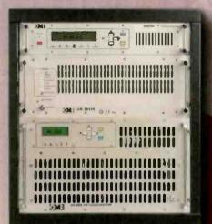
**EM 2000** is a 2000W FM transmitter made up of the EM 25 DIG exciter (or EM 20/30 exciter) and the AM 2000 FM amplifier. AM 2000 includes eight 300W high-efficiency MOSFET technology amplifying modules, fed by 2 independent switching power supplies, which are made to withstand the working conditions. The amplifying modules work independently thanks to a power combining structure that provides high isolation between them.
