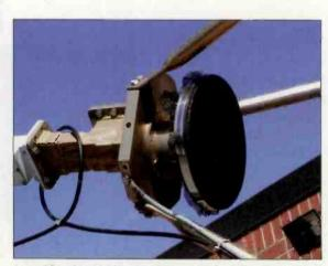
Bradford's Mylar LNB cover that he installed at WHMI.
