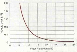
Figure 3. Rejection vs. broadband port loss
