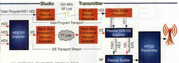
mon amplification, the transmitter needed to deliver 13kW of analog power and 621W of digital power to the antenna (which needed no adjustments). That is about 6 percent more digital power than would be required by MP1 mode – well within the capabilities of the HPX30 transmitter. There is also plenty of headroom to raise the HD Radio injection to as high as -10dB if needed in the future.
