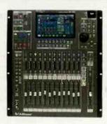
It features rapid recall of setups, 100mm motorized and touch sensitive faders, an 800x480 color screen, and dedicated knobs for EQ, pan and gain. It has digital patch-bays, built-in effects processors, 16 aux/mon sends, 8 matrices, 8 DCAs, 8 mute groups, built-in stereo recording/playback and support for LCR configurations.
