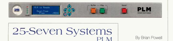
he Program Length Manager (PLM) from 25-Seven Systems is a 1RU time compression/expansion processor that can stretch or shrink audio programs in real time. It can be used to shorten the duration of programs, allowing additional material to be inserted with no loss of content, or stretch short programs so they precisely fill their allotted time slot. The PLM does this without pitch change, artifacts or glitches at various speed changes.
