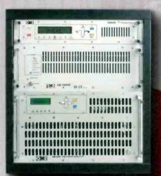
**EM 2000** is a 2000W FM transmitter made up of the EM 25 DIG exciter for EM 20/30 exciter) and the AM 2000 FM amplifier. AM 2000 includes eight 300W high-efficiency MOSFET technology amplifying modules, fed by 2 independent switching power supplies, which are made to withstand the working conditions. The amplifying modules work independently thanks to a power camplining struc ure that provides high isolation between them.
