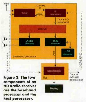
There are four underlying transport protocols used to encode the data received from a data client prior to application into the RLS transmission stream. When transferring synchronized images, the difference between the packet delivery methods can dictate how far in advance of the associated audio the image must be sent to ensure it is available for display when the associated audio arrives:
