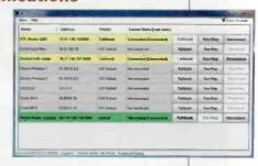
to maintain a one-way talkback connection to several Access Portable users in the field. While each of the users can monitor a talkback feed from the studio, a full-duplex connection can be initiated from the studio with any of the remote devices simply by selecting the two-way button.
