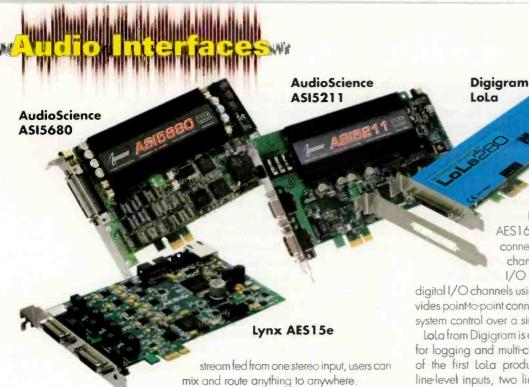
AusioScience also created the ASI5211, a PCle version of the ASI5111 card. It removes time-critical audio processing burdens from a PC, featuring two stereo record streams fed from either a balanced analog input or an AES/EBU digital input, four stereo play streams mixed to both a balanced analog output and and AES/EBU digital output, and a mic input. The analog I/O level has been in-
