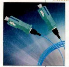
**SC Multimode:** Fiber Express Brilliance Field-Installable SC Multimode Connectors for 900 micron fiber termination enable fast, fool-proof and easy termination of a fiber. Terminations can typically be made in less than five seconds, with no termination tools required. Insert the fiber into the connector. Using the index finger, slide the connector's switch-like activator toward the fiber to be terminated to bring about the splice/crimp. Slide the boot on the connector body, and it's done.
