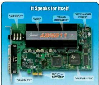
The ASI5211, Not another dumb card. With a microphone input, including a low noise pre-amp and 48V phantom power supply, on-board DSP. increased analog I/O level of +24dBu and a new GPIO that adds two opto-isolated inputs and two normally open relay outputs, the ASI5211 is one smart card. And considering it's priced the same as cards without all these features, it's one smart choice, too. For information, call +1-302-324-5333 or email salesasi@audioscience.com
