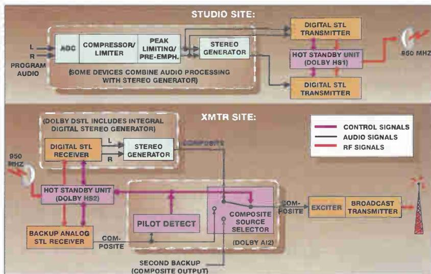
**Figure 1.** Hot-standby installations using digital STLs with analog backup must cope with discrete and composite audio signals. For fully automatic operation, the receiver must also sense whether the digital or analog system is using the STL channel. A pilot-detect circuit accomplishes the latter.
