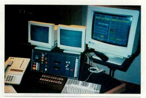
At WMC-AM in Memphls, an ENCO Systems' DAD486x network is used for live-assist daytime operation and overnight automation of the station's news/talk format. Seven DAD486x workstations and two file servers are linked via LAN, with separate monitors used for audio (touchscreen at right) and text (at center) displays. In this talk studio, a third monitor (at left) displays queued caller data.
