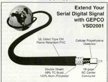
Gepco's Video Serial Digital cable outperforms traditional precision video cable because it has a larger center conductor and dielectric which means lower attentuation at higher frequencies. This enables you to make longer cable runs.
