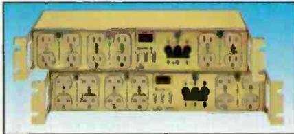
Rack mounted. Designed to fit standard 19" wide EIA STD. Standard and optional features including EMI/RFI filter, spike and surge suppression, 12 front panel mounted NEMA outlets, remote I/O ports, current protection up to 24 AMPS. Other features include three sections of four outlets either all switched or two switched and one unswitched, Multiple Time Delay® power-up/down, various current/voltage ratings.
