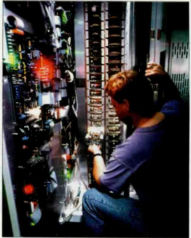
The solid-state design of this Harris DX series AM transmitter allows a single RF amplifier module to be used throughout the transmitter.
