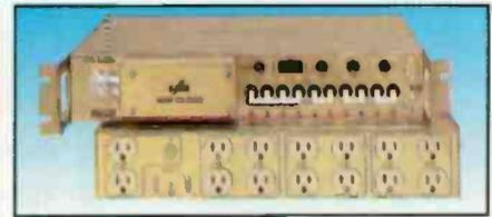
Rack mounted. 3-1/2" (2U) high. Depths from 8-1/2" to 14-1/2". Includes spike and surge protection, EMI/RFI filter, remote I/O connectors for power on/off, EPO and power-up of additional equipment down line; precision electromagnetic circuit breakers and power indicator lights. Options include Multiple Time Delay® power-up between sections, receptacle type and output voltages of 125 or 208 VAC. Designed to meet UL 1950 and CSA 22.2-950.
