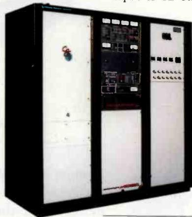
The Continental 816R series is an example of hybrid FM transmitter design. It combines a solid-state exciter and an IPA with a tube final stage for powers ranging from 21.5kW to 35kW.
