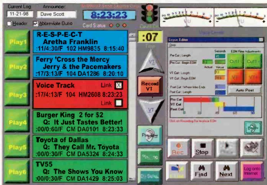
Here's Scott Studios' Voice Trax Via Internet (VTVI) software, shown with the optional Segue Editor. VTVI allows a distant announcer to pre-record a 4 hour show in about 15-20 minutes with nothing more than a Windows computer with an ordinary sound card, an Internet connection and a good microphone.
