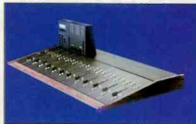
A 12-channel, low-profile control surface. Accepts up to 16 stereo inputs. Metering/monitor select panel can be mounted on the left or right side. Graham-Patten Systems builds the internal electronics. Input connections are XLR.
