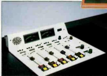
can be done without turning off the console. Flex configurations, three monitor sections, VU meters. Outboard audio engine allows for flexible DSP reconfiguring, factory support, short learning curve, low price point. Non-modular surface. DB connector I/O.
