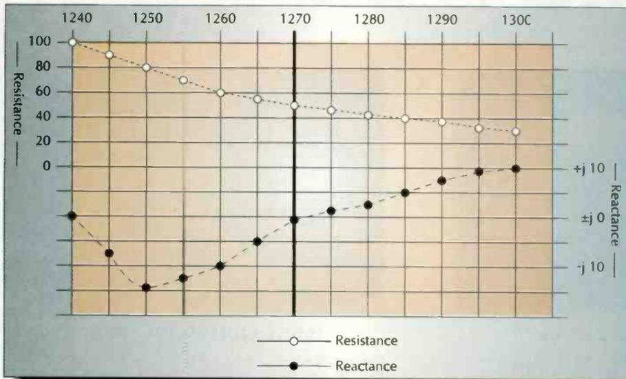
**Figure 2.** This figure shows a typical antenna base operating impedance chart of the type the FCC requires to be present in every AM station.
