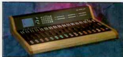
The second generation of this console (the DRC1000 is still available) offers 11 stereo inputs per audio processing unit (APU) with AES-3ID (75Ω) or analog connections. Seven stereo outputs are provided. Each channel has a five-band parametric equalizer and dynamics processing.
