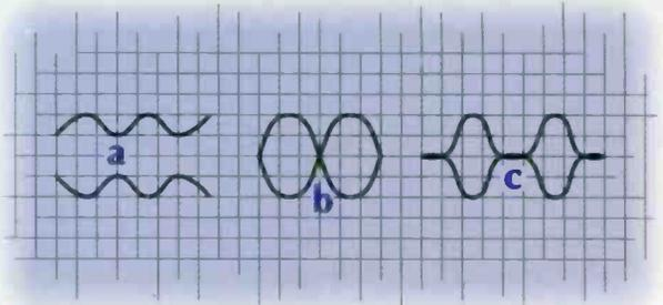
Figure 2. The AM carrier waveform with modulation.
