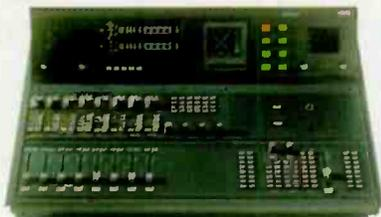
Vadis is a digital routing switcher that serves as the audio engine for the Vadis D.C. console. Inputs can be analog, AES3, ADAT or MADI format. Fully loaded, the system can handle 1024 inputs and 1024 outputs. Change configurations at the press of a button.
