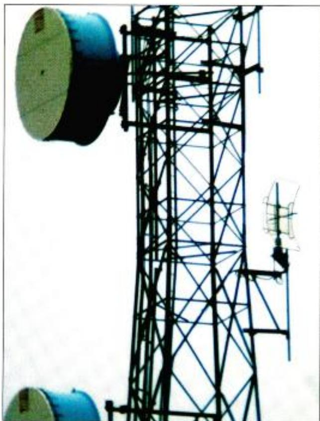
**The ATTC DOCR receive antenna had a direct line-of-sight view of the primary station 42 miles away. The antenna was mounted on a rotor to investigate the effects of antenna orientation and coupling in the DOCR antenna system.**
