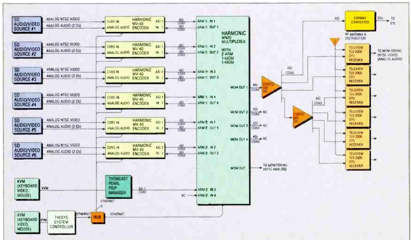
Paxson's WCPX-DT is multicasting six channels of programming in its allotted 6MHz. The station employs Harmonic encoding and multiplexing equipment, Evertz DAs and Thomcast's Pearl PSIP manager.
