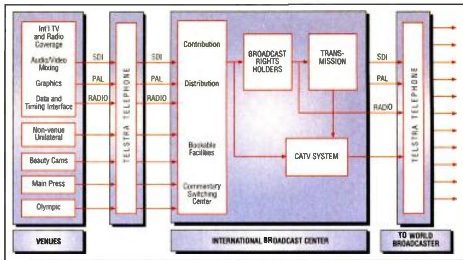
**Content flows from the various venues to the IBC, then from the IBC to the individual rights holders via Telstra fiber and codecs.**
