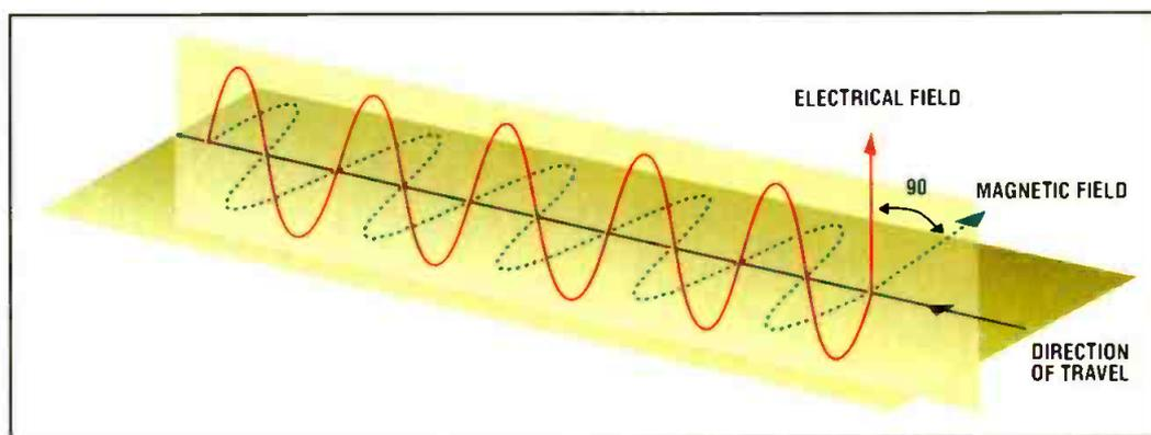
Figure 2. Electromagnetic waves travel as an electrical wave and a magnetic wave on two separate planes at a 90 degree angle.
