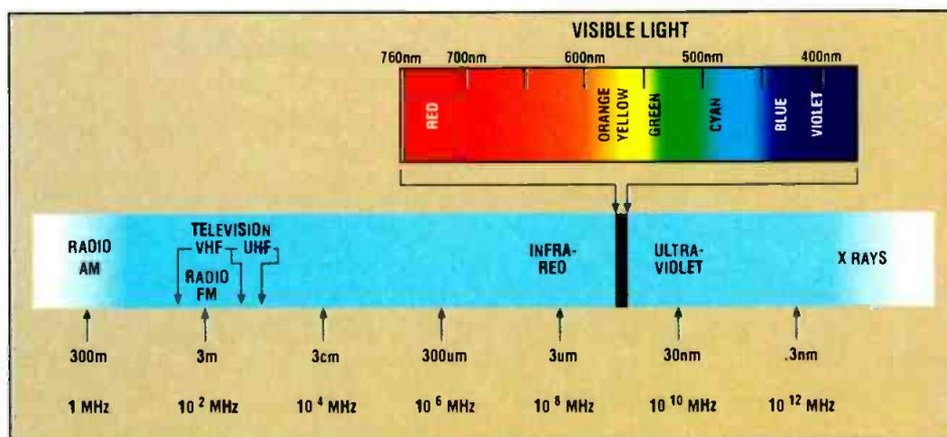
Figure 3. The spectrum of electromagnetic radiation includes the AM & FM radio bands, VHF and UHF television frequencies as well as visible light.
