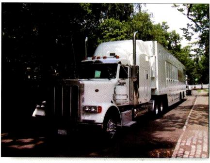
DX11 is a 53-foot production trailer with a 47-foot curbside expando that opens up an additional five feet.
