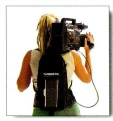
Tandberg Television introduces its Voyager Lite backpack ENG solution designed for wireless cameras. The system incorporates high-quality video encoding with an integrated DVB-T modulator/upconverter, providing 2.4 GHz RF output. The entire unit fits into a small pack and is carried on the cameraperson's back. Once attached to a wireless ENG camera, Voyager Lite turns the cameraperson into a moving broadcast station.
