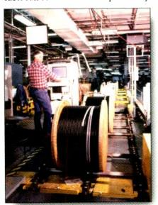
This roll of coax is being swept for return loss during the manufacturer's final quality control procedure. Photo courtesy CommScope.
