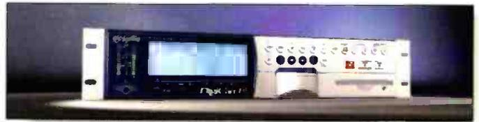
New networkable audio recorder operates at 16 or 24 bits and at all sample rates; features a large LCD display; files are compatible with earlier Digicarts; editing tasks include trims, fades and level adjustments.
