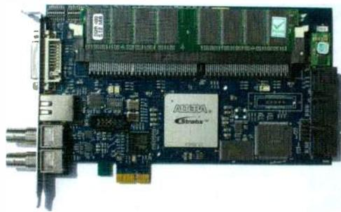
Figure 1. Fairlight's CC-1 board with Altera's Stratix II GX is 4in x 8in and replaces eight QDC boards.
