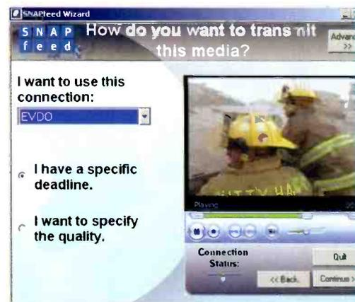
The SNAPfeed interface makes it easy for journalists in the field to contribute footage to an ingest server in an ENPS newsroom via a standard IP network connection.
