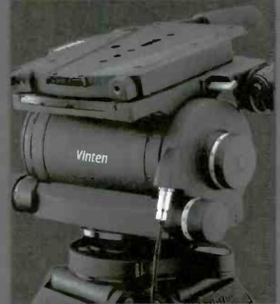
The **Vector 950 Active** comes complete with a standard four bolt base, single telescopic pan bar and wedge adapter. It offers an increased capacity of up to 120kg/265lbs providing perfectly balanced tilt. By combining the characteristics of the TF drag control with infinite perfect balance adjustment, the effort needed to control the effect of a heavy, moving camera payload remains constant, predictable and minimal— not a major distraction.
