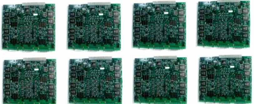
Figure 2. The Fairlight QDC board measures 10in x 10in. Altera's Stratix CC-1 replaces these eight boards.
