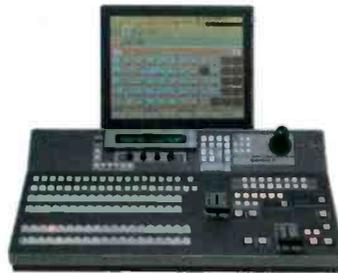
Digital switcher includes frame synchronizer for every input, up to 16 SD inputs and outputs, six keyers and six channels of 3-D DVE; allows 120 seconds of uncompressed video recording and provides two channels (key/fill) with simultaneous playback for video insert, CG wipe or slow-motion playback; users can add 2-D DVE in every input, delivering up to 32 DVE channels.
