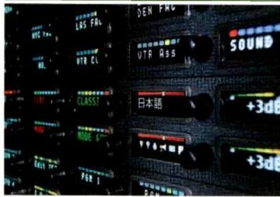
Control key panel for Artist digital matrix intercoms; features high-res color OLEDs, with 65,000 colors and a resolution of 140 dpi; the new displays provide readability and can show up to eight highly detailed characters of up to 24 x 24 pixels, ideal for displaying icons and Asian characters; definable marker colors for the keys complete the labeling options and provide instant function identification and signalization, e.g. for incoming calls.
