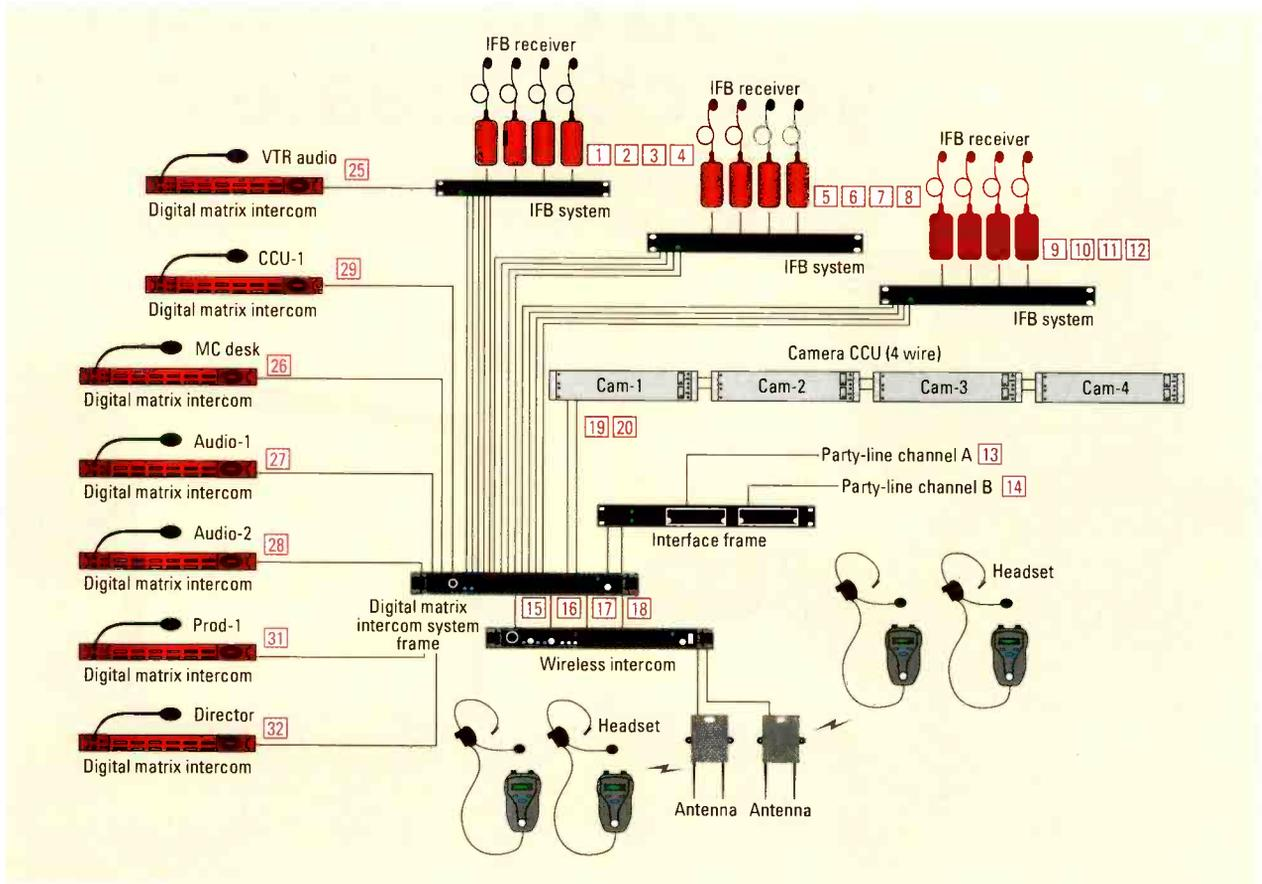
Figure 2. A matrix system with a wireless component
