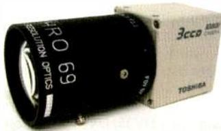
High-quality 3.5mm lens is designed for use with the latest 1/3in miniature three-CCD HD cameras; features 3.5mm focal length, 69-degree horizontal angle of view, F2.2-F16 aperture range, back focus, a special bump cover to protect the lens front and 40.5mm filter thread adapter option; includes stainless steel locking screws for aperture and focus adjustment, as well as spare lens caps.
