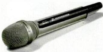
Handheld transmitter provides sound engineers with expanded switching bandwidth of up to 184MHz; features adjustable sensitivity from 40dB to zero in 1dB steps and a three-position low-frequency filter; operates in low intermodulation mode, which increases the number of usable channels in crowded RF environments, standard 10mW mode to extend operating time and 50mW to increase the transmitter's range.
