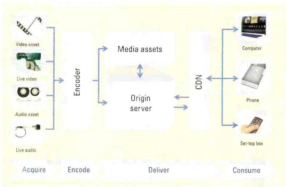
Figure 1. A basic streaming workflow includes acquisition, encoding, delivery and consumption.
