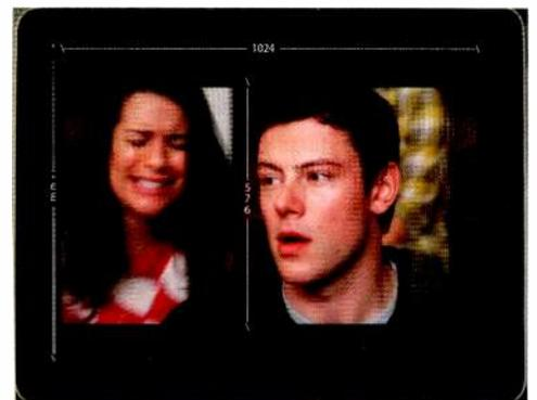
Figure 1. A 720p video played on an Apple iPad is scaled down to 1024 x 576 with letterboxes on top and bottom.
