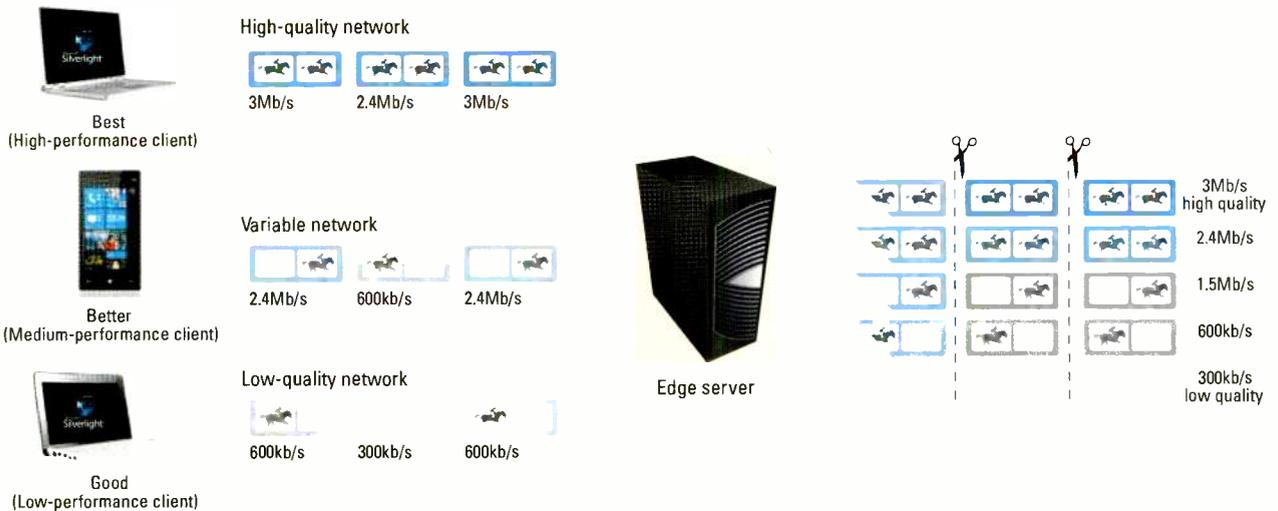
**Figure 2. Microsoft IIS Smooth Streaming can adapt to changing network conditions by varying the quality of the stream.**
