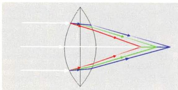
**Figure 1. If chromatic aberration exists, meaning all three images do not converge in the same plane, adjustments could be made. But new modern lenses have fixed imagers, so the lens must provide precise focus.**
