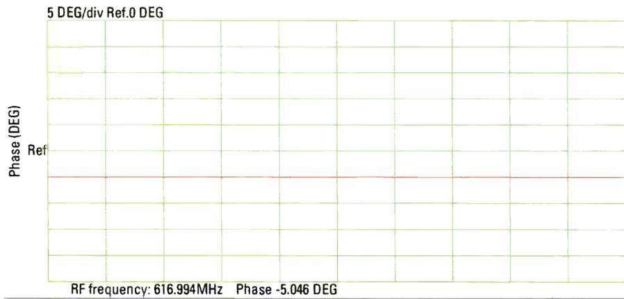
Figure 9. Final measured phase difference at midband Channel 38
