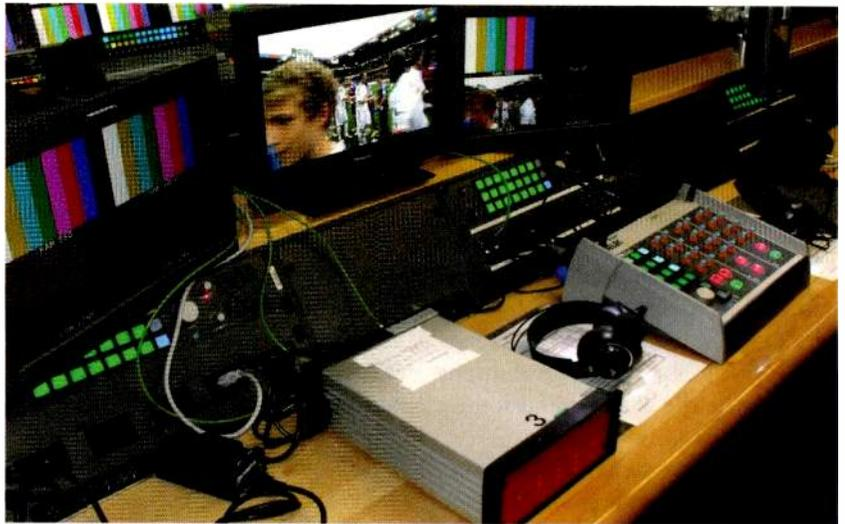
**Nevion's FlashCase portable housing connects camera sites to production trucks or other facilities through a lightweight optical fiber cable.**
