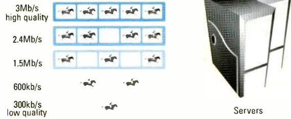
**Step 4 Consumption:** The edge server delivers the most appropriate stream to each client. Stream quality depends upon both the client and the network.
