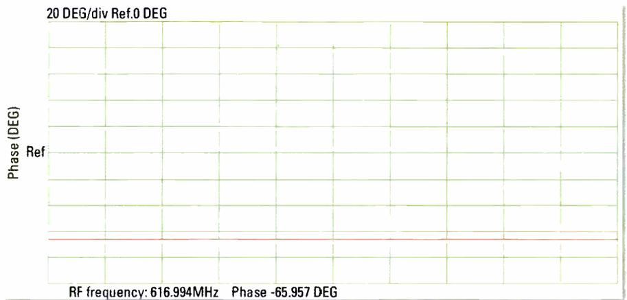
Figure 6. Initial measured phase difference at midband Channel 38
