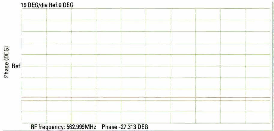
Figure 5. Initial measured phase difference at midband Channel 29
