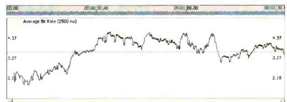
Figure 4. This frame-rate graph from Inlet Technologies Semaphore shows lower data rates during the start of the test clip, which begins with 30 seconds of low-motion talking head footage, and then higher data rates for the higher-motion content that follows.
