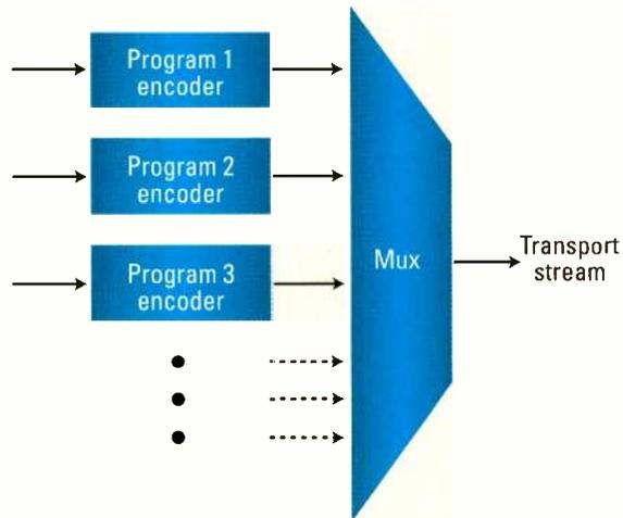
Figure 1. Transmission multiplexing involves the generation of transport streams. Within these streams, the various programs are compression encoded.
