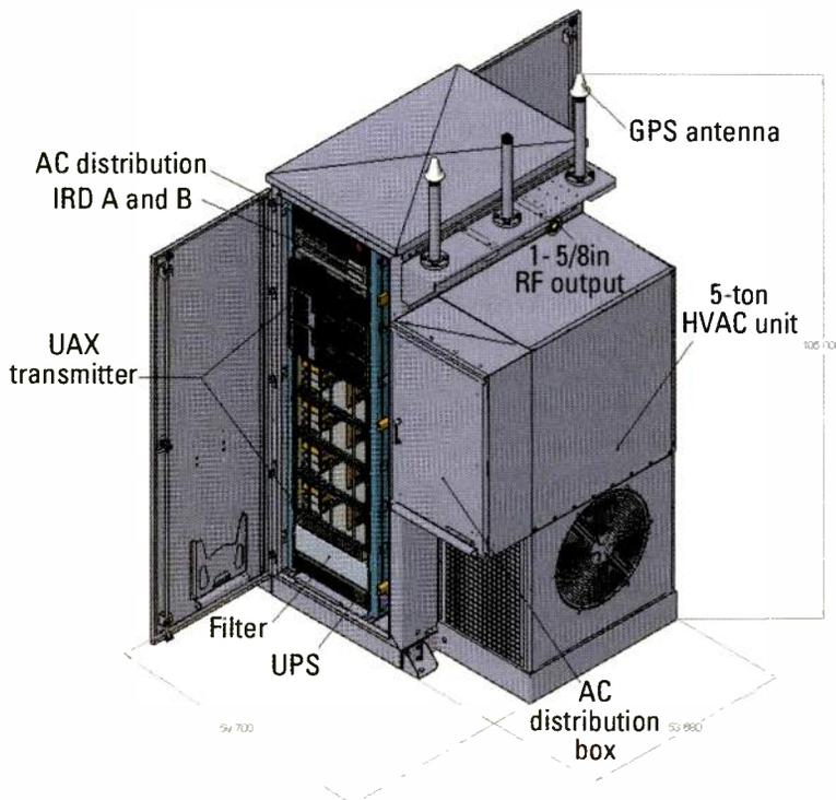
**This diagram breaks down the design of an outdoor enclosure featuring a Harris Maxiva UAX air-cooled transmitter. Note the antenna mounting options on the roof and how the AC distribution cycle pulls air from the top of the enclosure, creating a continuous airflow pattern that maintains operational efficiency.**
