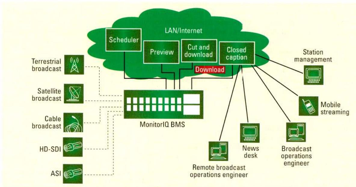
Figure 1. Digital Nirvana's MonitorIQ BMS integrates with other broadcast operations systems. Staff can access the BMS using any Web-enabled device from any location.
