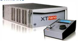
Entry-level replay and live slow-motion server for live broadcasters and OB facilities; housed in a 4RU chassis offering four configurable channels (two cameras IN and two OUT for preview and program control, or three IN and one PGM) and native support of DVCPRO HD and DVCPRO 50; dual Gb/s Ethernet networking provides faster than real-time file transfers.
