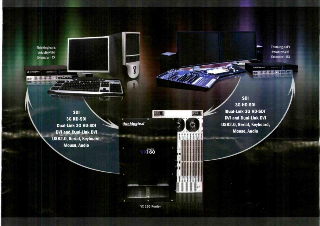
Route and switch virtually any desktop device up to 40 kilometers away from the controlling computer.
