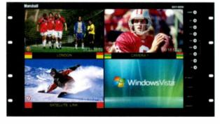
Full-resolution monitors with IMD; available in different sizes; allows viewing of four different inputs at once with three different layouts to choose from; does not require external under monitor display; supports the following protocols: Image Video, NVISION, TSL and MEI; offers a full-resolution 1920 x 1200 display; new unique RotoMenu feature enables fast, direct and easy menu navigation.
