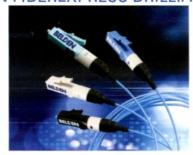
Enables fast, fool-proof, easy fiber termination in the field with no tools required; built-in activator tab performs the fiber splicing and crimping action in one simple motion; users can verify proper connection using an external laser light source, which can be clearly seen through the connector's window, offering immediate termination assurance; available for 900μm LC (OM1, OM2, OM3 and OS2).
