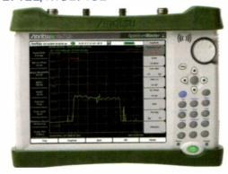
Eliminate multiple test sets; can be configured to include two-port transmission measurements, spectrum analysis, interference analyzer, channel scanner, gated sweep, CW signal processor and power meter; a GPS receiver can be added to both models; feature AM/FM/PM analysis capabilities.
