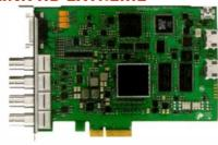
Now includes dual link and 3Gb/s SDI for 4:4:4 quality, and a new hardware downconverter for simultaneous HD and SD playback; connects to SDI, HDMI, component analog, NTSC/PAL and S-video equipment for capture and playback, while instantly switching between SD, HD and 2K.
