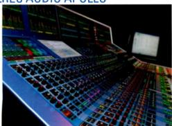
Relies on Bluefin2 for processing; at 48kHz, Bluefin2 gives Apollo up to 1020 channel processing paths, 128 program busses, 96 IFB/track outputs and 48 auxiliaries; at 96kHz, Apollo affords 510 channel processing paths, 64 program busses, 48 IFB/track outputs and 24 auxiliaries; features a second dynamics section in each channel, more than 70 minutes of assignable delay and three independent APFL systems for multiple operator use.
