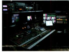
Designed to meet the demand for HD production facilities in hard-to-access production spaces for sports, entertainment and reality TV; features lightweight HD technology, an LCD monitor wall, working positions incorporated into custom equipment racks and optimized rack design and mechanics; can be set up quickly, is flexible and can handle many different types of production requirements.
