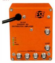
A 1 x 4 3G/HD/SD-SDI distribution amplifier; provides cable equalization, reclocking and distribution; features high performance and low cost; can distribute 3Gb/s, 1.5Gb/s and 270Mb/s data rates; can equalize 400m at 270Gb/s, 200m at 1.5Gb/s and 140m at 3Gb/s of 1694A coax cable; non-SMPTE data rates may be distributed by using the internal reclock enable switch; can pass data rates from 143Mb/s to 2.97Gb/s while in bypass mode; ASI-compliant at 270Mb/s; a separate loop output is also provided.
