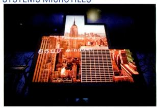
Can be stacked and clustered like building blocks to create display walls of any shape or scale; offer superior color and image reproduction, wide viewing angles and only 1mm gap between tiles; based on LED and DLP technologies; rated at 65,000 hours to half brightness usage or nearly 7.5 years of continuous operation; feature a screen size of 16in x 12in x 10in; require 2in of minimal clearance for rear ventilation; include built-in sensors that automatically perform color calibration.
