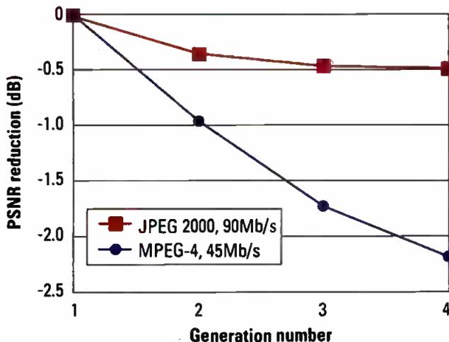
**Figure 4. Multigeneration encoding**
