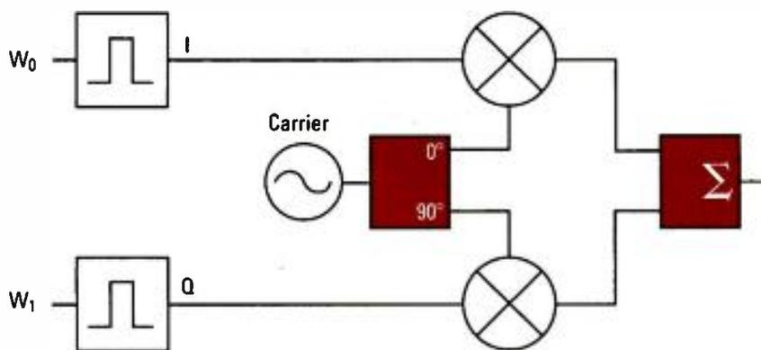
Figure 1. QAM modulator
