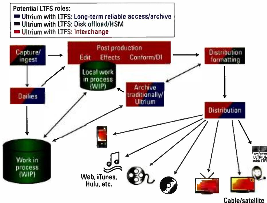
**Figure 1.** LTO tape is already firmly established in the media production environment. For production, LTFS efficiently supports several important requirements such as camera media reuse, backup, transport, direct access to data and archiving.
