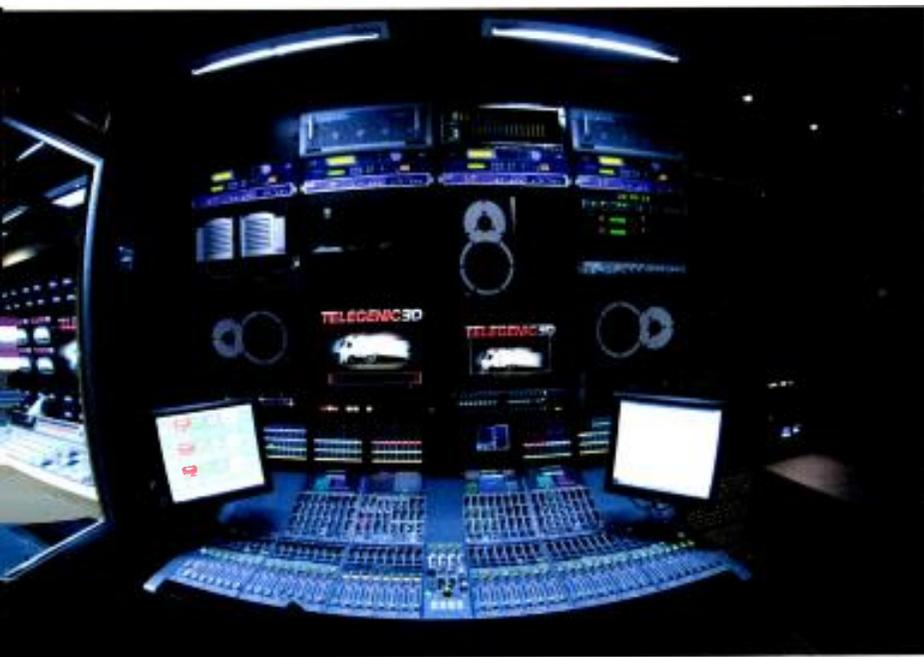
Shown here aboard a Telegenic OB truck, the Calrec Apollo console allows users the option to output LtRt phase-encoded signals directly from the console's main outputs.
