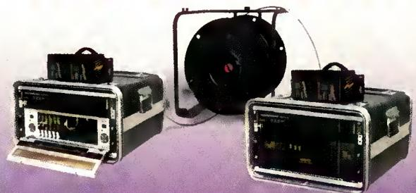
**Complete Mobile Fiber Optic Systems:** Includes transit cases, frames, TAC-4 fiber optic cable with hermaphroditic connectors, cable reel, and an AC/DC Changeover unit (7700-PCD).
