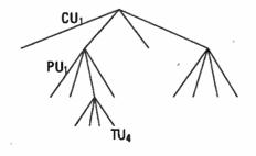
Figure 2. With HEVC, video frames are divided into a hierarchical quad-tree coding structure that uses coding units, prediction units and transform units.
