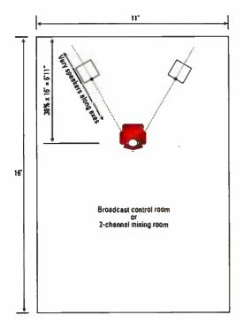
Figure 1. This shows idealized placements for the loudspeakers and prime listening seat in a room used mainly for stereo playback.
