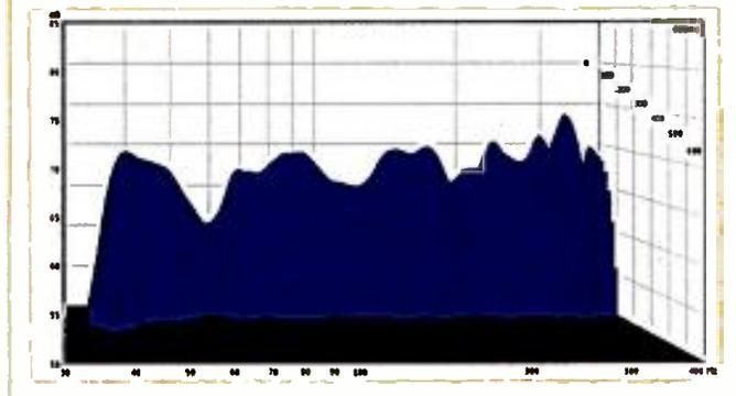
Figures 3 and 4: These graphs are derived from the same measurement data as Figure 2, but they show each peak's decay time, as well as amplitude. The red graph shows the room when untreated, and the blue graph is after adding bass traps.
