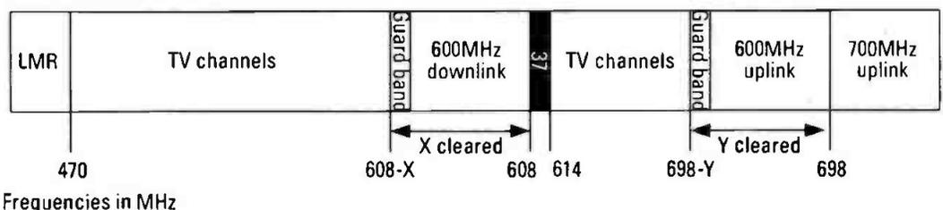
Figure 1. FCC proposed repack plan, 600MHz band
