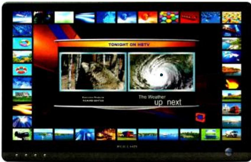
**Figure 1.** Because a channel-in-a-box system has graphics, automation and DVEs, squeeze backs with “coming up” text are based 100 percent on the playlist metadata. There is no need to build and import separate graphics.
