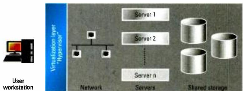
**Figure 2. Using virtualization, a single server, or groups of servers, may be set up as multiple VMs. The Hypervisor abstracts the VMs from the underlying hardware (host server), allowing the creation of multiple VMs that can use the available hardware resources.**
