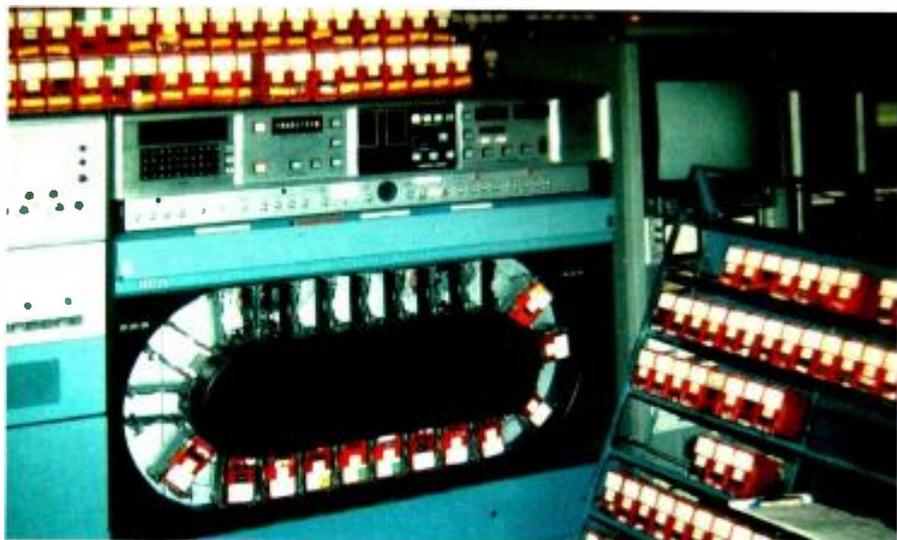
In the early 1970s, the RCA TCR-100 was 2600lbs of state-of-the-art station automation, requiring three 30A 120V circuits and engineers who knew how to fix it. Photo courtesy television.crossware.com.au
