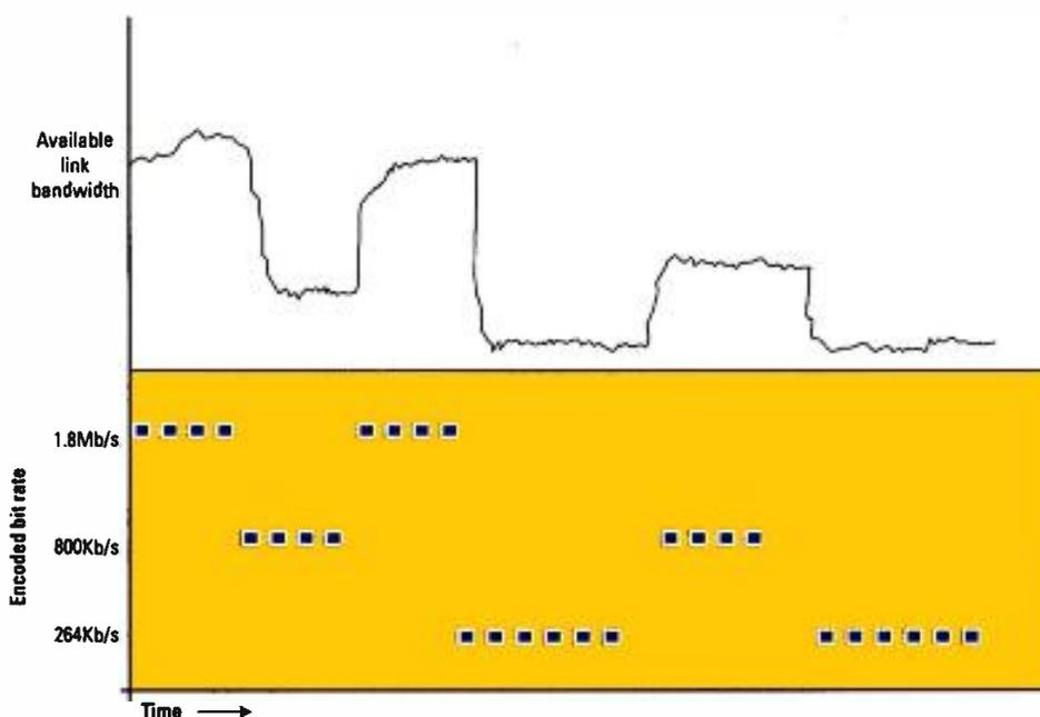
Figure 1. As available link bandwidth changes, the receiver requests content encoded at lower or higher bit rates.
