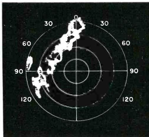
Figure 7. Indicator Display, 20 Mile Range, Contour
