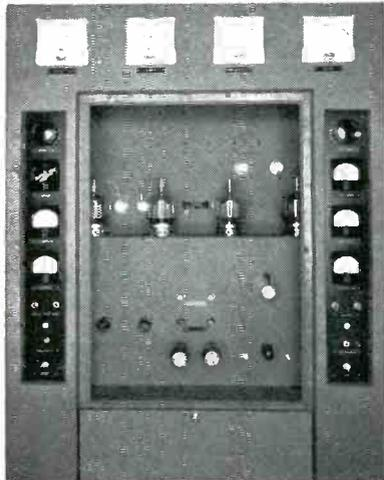
All audio and R.F. tubes are removable from upper door. Each critical circuit is separately metered.
