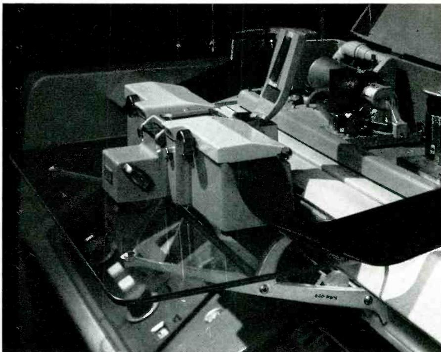
Closeup view of videotape splicer mounted on front of VTR console directly above control panel.
