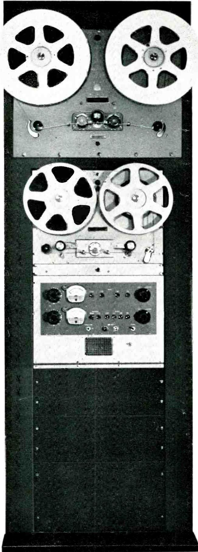
With the growth of special program services offered by broadcasters the need for automatic programming equipment is increasing. A system offered by Programatic Broadcasting Service in conjunction with a program service provides eight hours of operation per machine and by using three machines it is possible to program continuously for twenty-four hours. Announcements, which are recorded separately, are automatically injected into the program.
