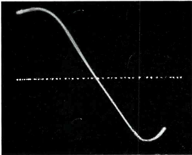
Fig. 3—Correctly adjusted discriminator or ratio detector produces this type of "S" curve. With a variable marker oscillator the length of the linear slope can be measured. It should be at least 200 Kc. for low distortion as well as for minimum demodulation of the subcarrier audio.
