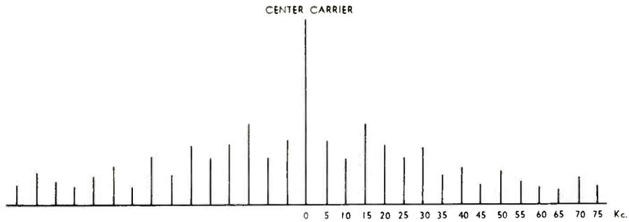
Figure 1—With 5000 cps modulation on the FM transmitter, sidebands are generated at intervals of 5 Kc. above and below the carrier. Audio tones of other frequencies will produce sidebands spaced in accordance with the frequency of the tone. The amplitude of the applied tone determines the extent of the deviation and the amplitudes of the individual side carriers.
