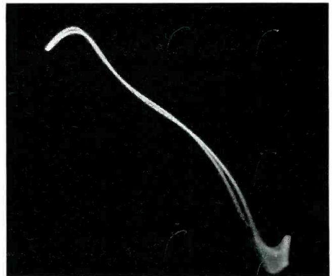
Fig. 6—With a typical misaligned discriminator such as this, there is no way of tuning in a station so that the subcarrier sidebands will balance each other. As a result, unwanted demodulation of the subcarrier will be heard along with the regular main channel program.
