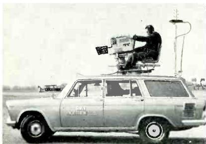
Fig. 1. Auto-top camera used in Italy.
