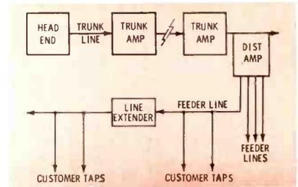
Fig. 4. Simplified system block diagram.
