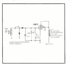
broadcast begins, a sample of the audio from the output of the line monitor amplifier is stepped up by the input transformer and rectified by a half-wave doubler, charging the 5-mfd filter capacitor and cutting off the 12BY7. This allows the relay to drop out and starts the tape deck
