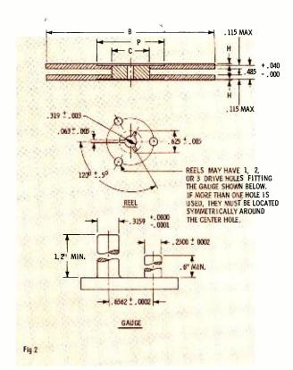
Fig. 2. Dimensions specified in Standard for NAB Type B reels.
