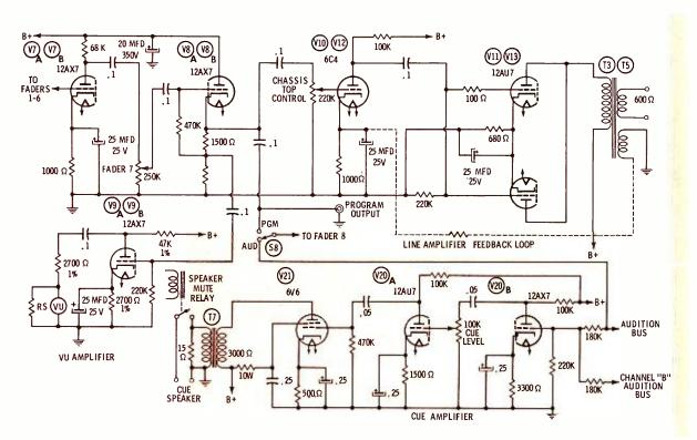
Fig. 5. Schematic diagram shows circuit arrangement and parts values of cue amplifier and one of the two-main channel amplifiers.
