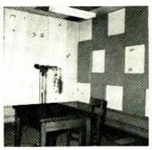
Fig. 4. Treatment of surfaces in small studio gives desired sound properties.
