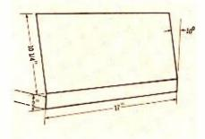
Fig. 8. Dimensions for bending the panel.
