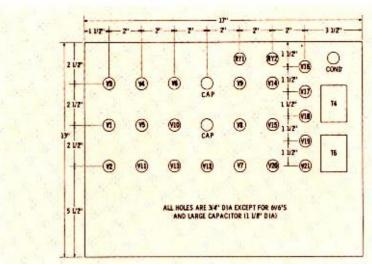
Fig. 9. Typical tube and transformer layout for the portable stereo consolette.
