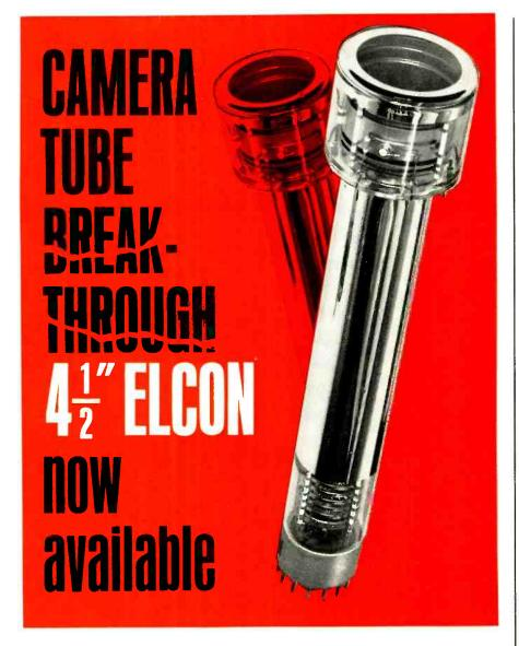
Long-Life, High Performance Television Camera Tube. An entirely new principle of operation, perfected by English Electric Valve, provides improved performance and increases tube life 3 to 4 times that of previous image orthicons.
