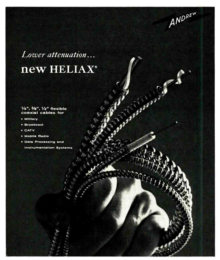
These new air and foam cables offer lower attenuation in small physical sizes. Type FH1,  $\frac{1}{4}$ " Foam HELIAX has 30% lower attenuation, 60% smaller size and 50% less weight than RG8/U. The copper inner and outer conductors assure optimum electrical performance with long life reliability. Available in long splice free lengths with or without polyethylene jacket.
