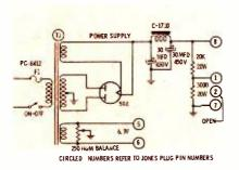
Fig. 7. Circuit of outboard power supply.
