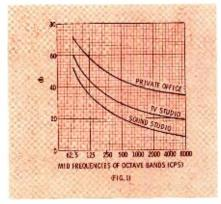
Fig. 1. Noise-rating curves (Kosten and Van Os) for three different environments.
