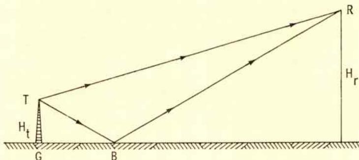
Fig. 2. Signal paths where transmitting antenna is below receiving antenna.
