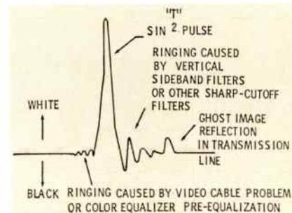
Fig. 7. Special graticule on waveform monitors measures sin<sup>2</sup> and bar pulses.
