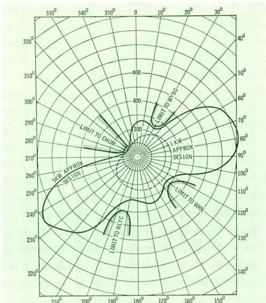
Fig. 3. Calculations show maximum possible radiation in protected directions.
