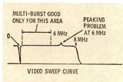
Fig. 5. Analysis of video sweep curve shows limits of multifrequency burst.
