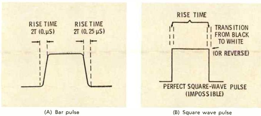
Fig. 4. Comparative evaluation of bar pulse and theoretical square wave pulse.
