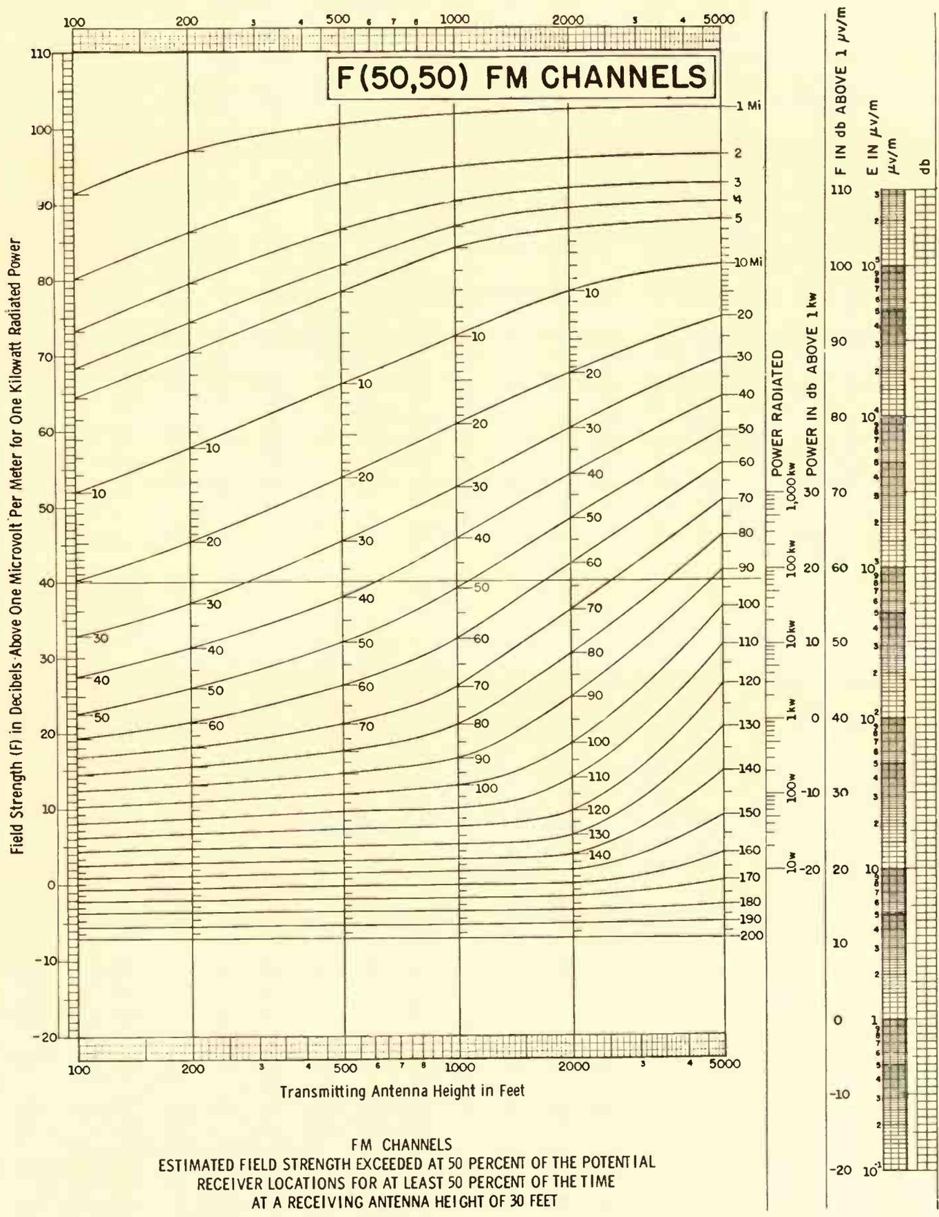
Fig. 1. Curves for predicting FM field strength. For below average terrain conditions use receiving antenna height.
