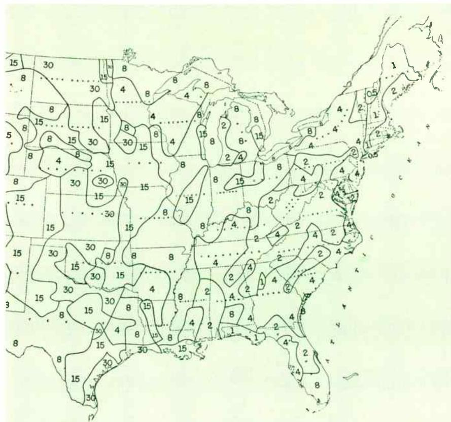
Fig. 4. FCC's Figure M-3 is simplified form of Figure R-3 for soil conductivity.
