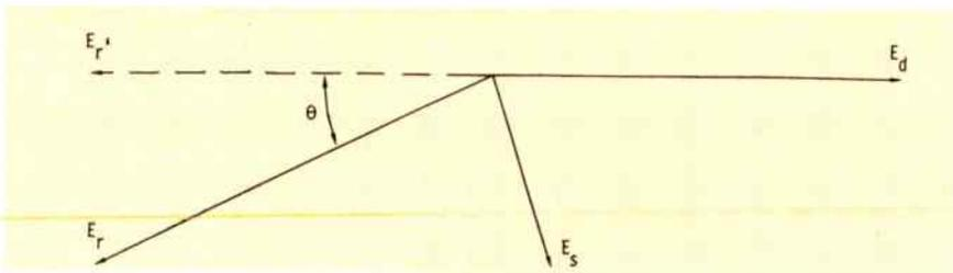
Fig. 3. Vector analysis of direct and reflected signals shows phase difference.
