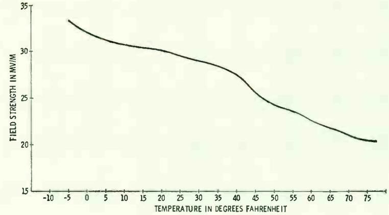
Fig. 2. Calculations indicate a relationship between signal strength and temperature.
