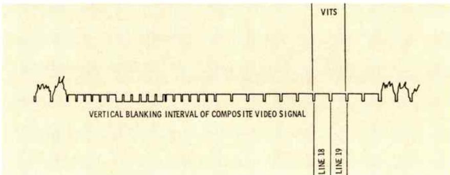
Fig. 1. Vertical blanking interval shows position of VITS on lines 18 and 19.
