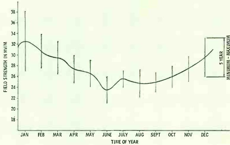
Fig. 1. Measured field strength at various times of year shows extremes of variation.
