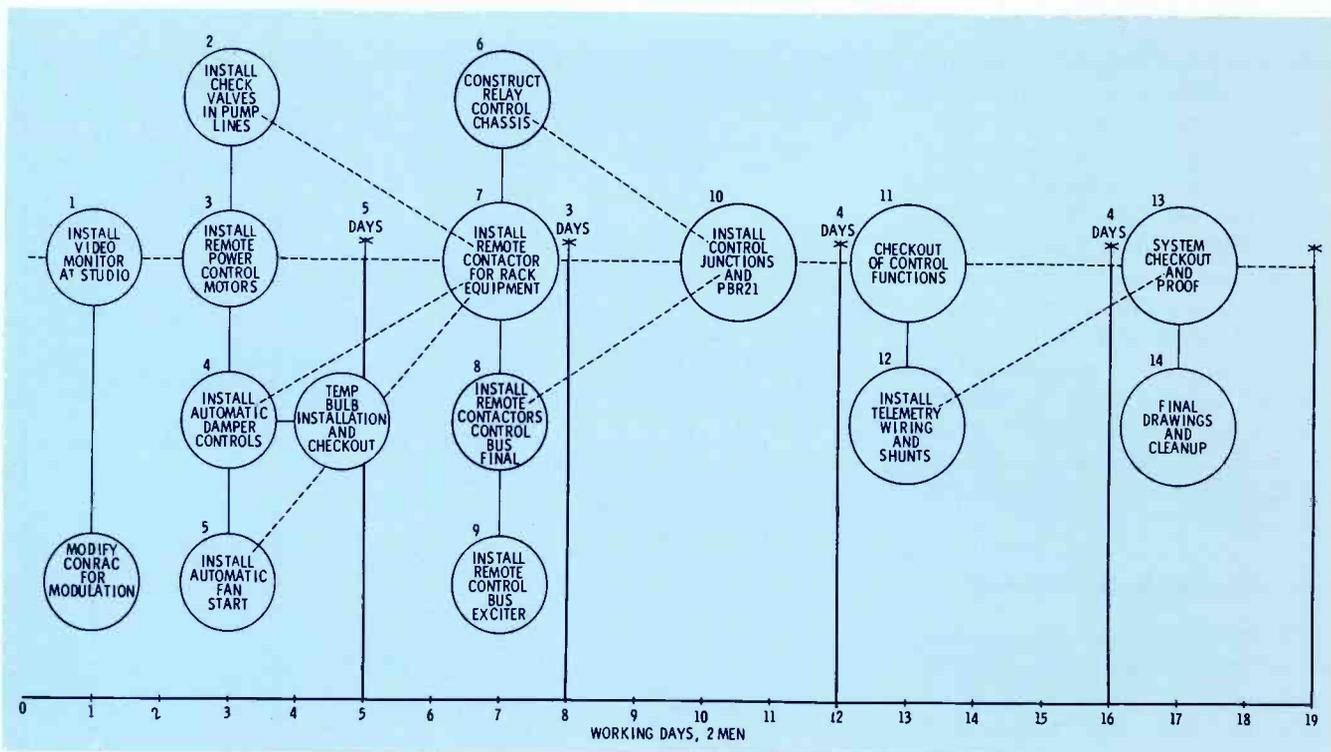
Fig. 4. Periodic Evaluation Review Technique (PERT) shows how work is accomplished in job versus time sequence.
