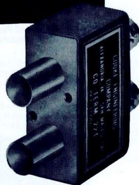
COTERM® provides the broadcast engineer with a new standard of dependability. With COTERM you have normal-through coaxial circuits without the use of patchcords. When the load side is patched the source is terminated automatically in the proper impedance.
