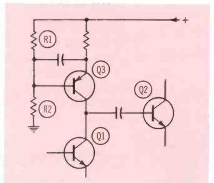
Fig. 8. Electronic choke replaces  $R_{L1}$ .
