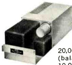
**ALTEC 9550A POWER SUPPLY** can power up to fifteen 9470A Amplifiers at full output. Entirely solid-state. External sensing circuit insures that output voltage will remain constant regardless of line voltage fluctuations. Under full 2 amp load, output ripple and noise is only 200 microvolts rms. 3"H x 3 3/8"W x 11 3/8"D.
