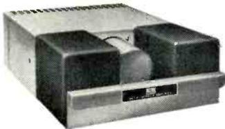
**ALTEC 9476A MONITOR / CUEING AMPLIFIER** is a fixed-gain plug-in unit with 8-watt output (+39 dBm) at less than 0.5% THD, 25-15,000 Hz. The all-silicon transistor amplifier features high gain, low noise and frequency response of  $\pm 0.5$  dB, 20-20,000 Hz. **Input Impedance:** 10,000 ohms (balanced). **Source Impedance:** 300 to 10,000 ohms. 3"H, 3 1/8"W, 10 3/4"D.
