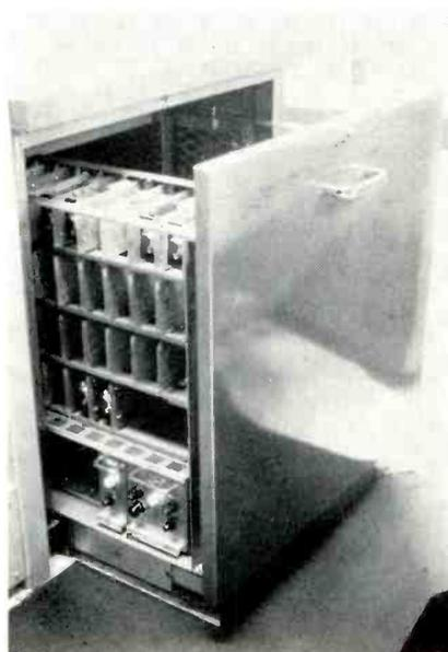
Fig. 2. Pull-out chassis at desk ends contain the solid-state circuit modules.
