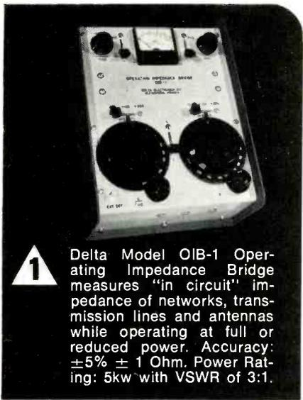
**1** Delta Model OIB-1 Operating Impedance Bridge measures "in circuit" impedance of networks, transmission lines and antennas while operating at full or reduced power. Accuracy:  $\pm 5\% \pm 1$  Ohm. Power Rating: 5kw with VSWR of 3:1.
