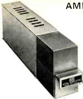
**ALTEC 9470A AMPLIFIER** can serve as preamp, line, booster, or program amplifier with no internal changes. All-silicon transistor circuitry delivers 0.5 watt and may operate continuously at 85°C without derating. **Frequency Response:**  $\pm 0.5$  dB, 20-20,000 Hz. Less than 1% THD, 20-20,000 Hz, with +27 dBm output. **Noise Level** (unweighted, 10-25,000 cycle band-pass):
