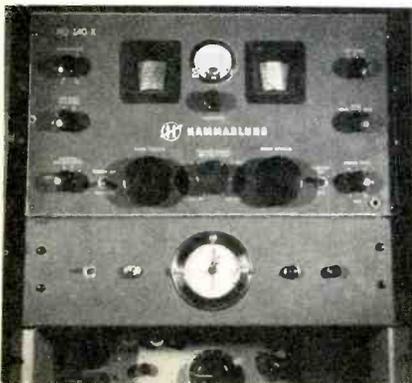
Fig. 4. Alarm uses thyatron, clock.
