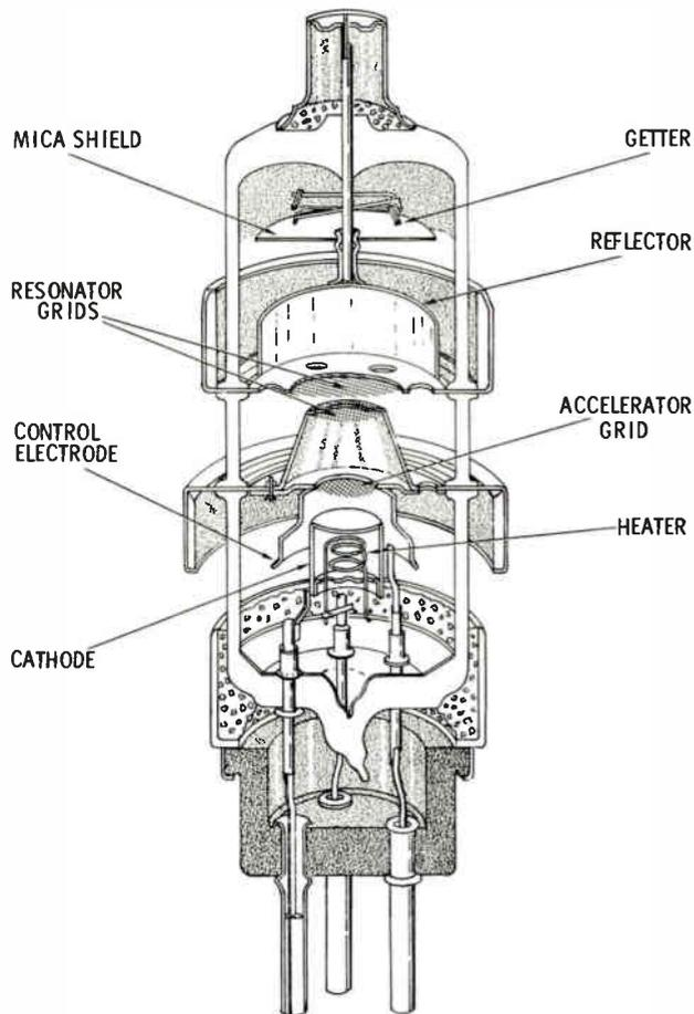
Fig. 4. A cutaway of an external-cavity reflex klystron.
