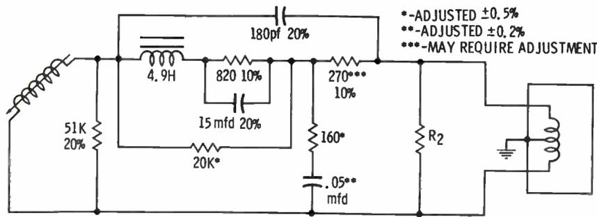
Fig. 4. The completed RIAA equalizer. Values and tolerances are correct for an 18-inch, low-capacity, shielded cable from the tone arm to the equalizer.
