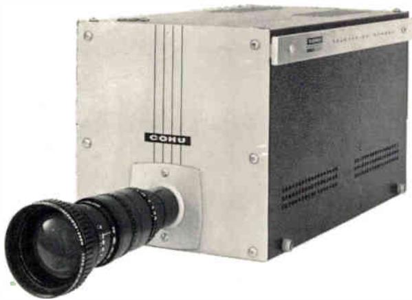
**IT'S A CCTV CAMERA** – completely self-contained. Just add a single coaxial cable to any video monitor and it's ready to operate. Want high resolution? Plug in one of four optional integrated-circuit sync generator boards for 525-, 729-, 873-, or 945-line scan patterns.
