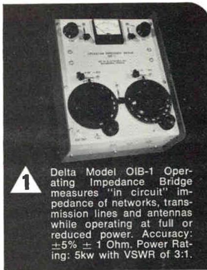
**1** Delta Model OIB-1 Operating Impedance Bridge measures "in circuit" impedance of networks, transmission lines and antennas while operating at full or reduced power. Accuracy:  $\pm 5\% \pm 1$  Ohm. Power Rating: 5kw with VSWR of 3:1.
