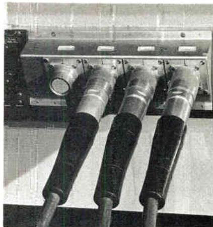
Fig. 9. Camera cable is terminated in studio terminal box with angled front.
