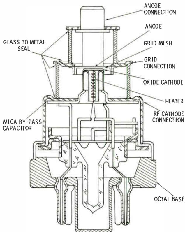
Fig. 1. The lighthouse tube minimizes transit-time effects by extremely close spacing of cathode, grid, and anode.
