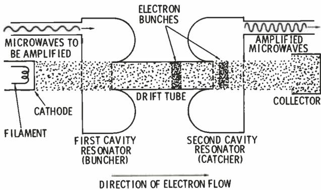
Fig. 2. Basic elements of a two-cavity klystron amplifier.
