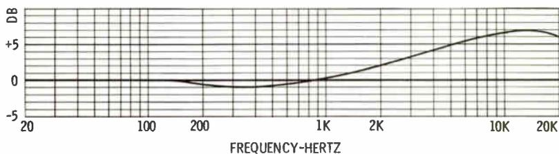
Fig. 1. Response curve of a commercially available, equalized preamplifier.
