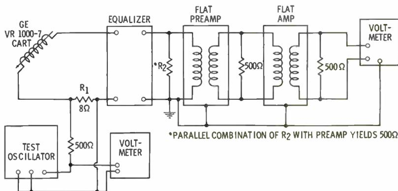
Fig. 2. Setup for measuring overall response of the equalizer and amplifier.
