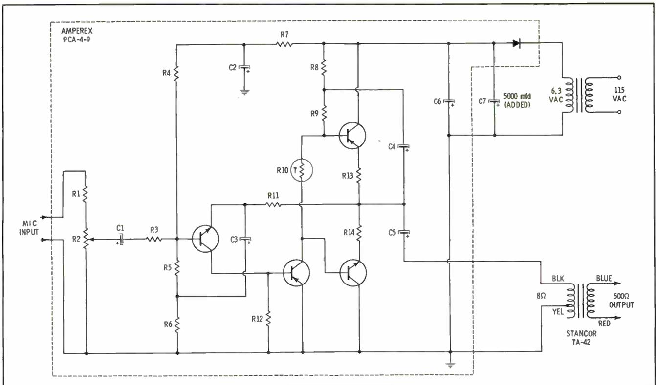
Fig. 1. The solid-state "call-letter-sign" amplifier is based on a commercially available unit, with modifications indicated.
