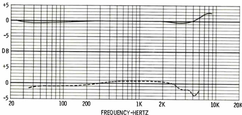
Fig. 5. Deviations from the RIAA recording curve of two "standard" records.
