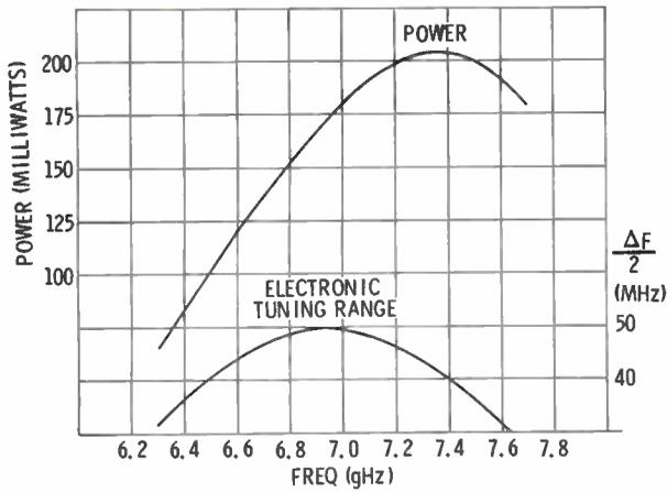
Fig. 6. These curves show the power output as a function of mechanical tuning and the electronic-tuning range of a typical reflex klystron which operates in the lower X band.
