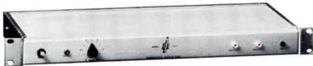
The TC1 Clamping Amplifier employs tip clamping to remove low frequency signal deficiencies without disturbing burst and other chrominance information in or about back porch levels. The clamped stage utilizes a field effect transistor driven by a balanced bridge circuit. This advanced design technique produces highly effective and stable clamping. The TC1 Clamping Amplifier sells for \$325.00 F O B Nashville.
