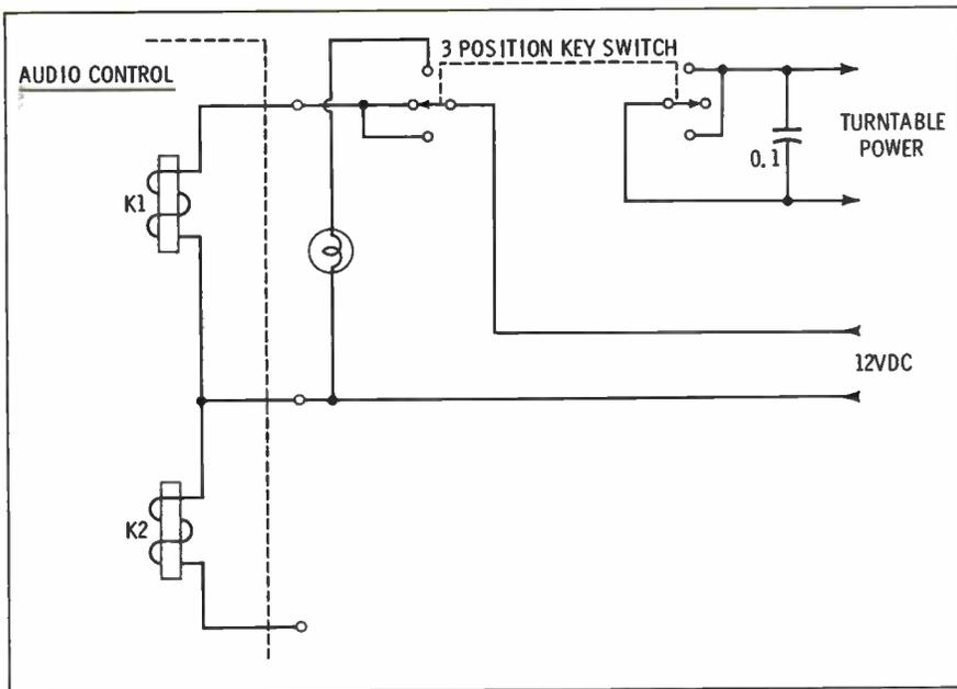
Fig. 2. Alternate arrangement uses key switches to control power and audio.
