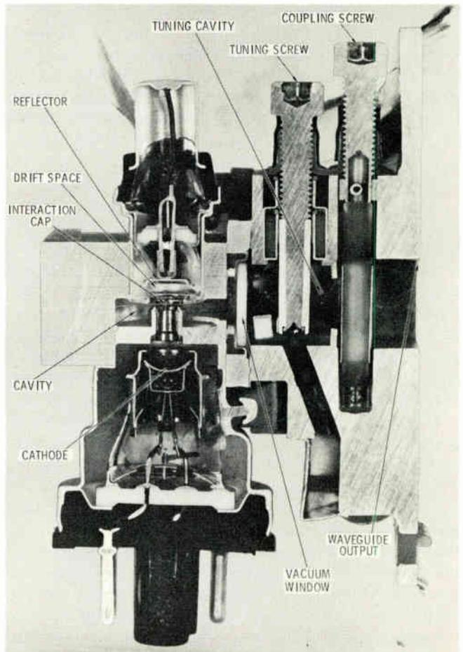
Fig. 8. A reflex klystron tuned by a cavity tuner. Most of the modern external-cavity klystrons are of this type.
