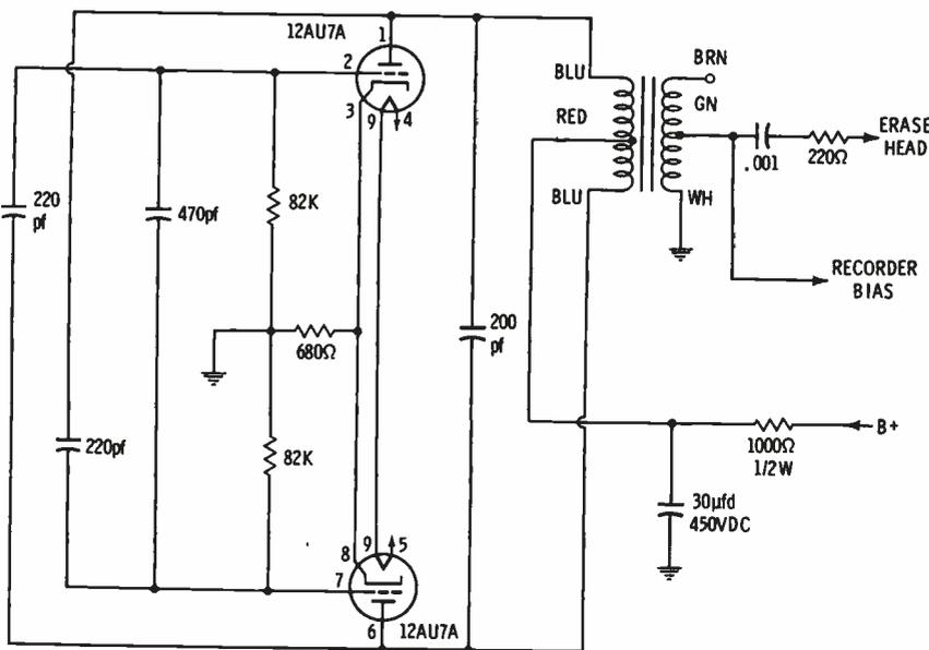
Fig. 2. This push-pull, 70-kHz bias/erase oscillator replaces the original.
