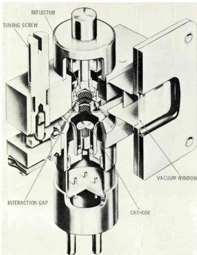
Fig. 7. Cutaway illustration of a reflex klystron. Tuning is accomplished by varying the width of the interaction gap.
