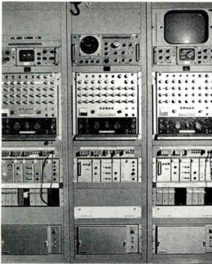
Fig. 4. Vertical aperture equalizers, in the right racks, are on order for all.
