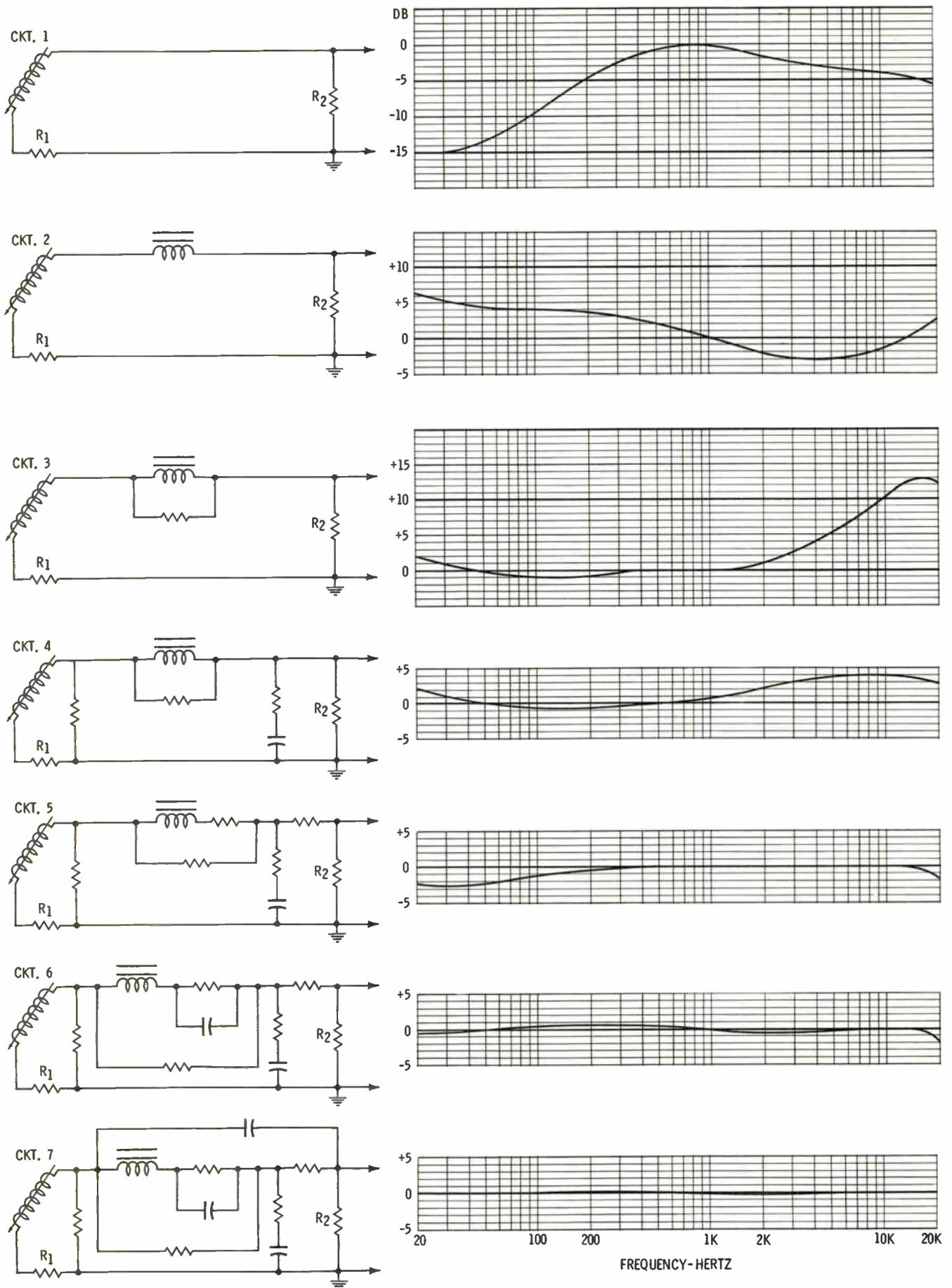
Fig. 3. Seven steps in the evolution of the equalizer. The curves show the output with a standard RIAA input.
