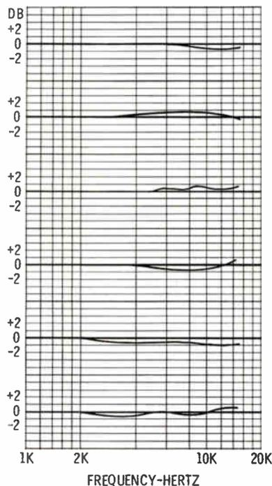
Fig. 6. Response curves of six VR 1000-7 cartridges selected at random.
