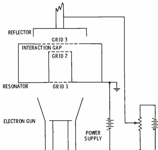
Fig. 3. Simplified diagram of a reflex-klystron oscillator.
