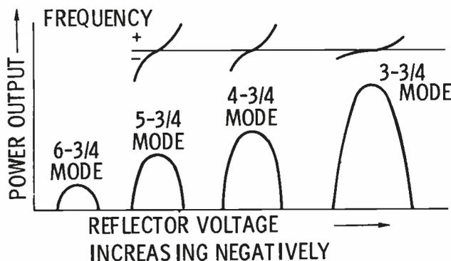
Fig. 5. Reflector-mode graph showing power vs reflector voltage and frequency vs reflector voltage for each mode.
