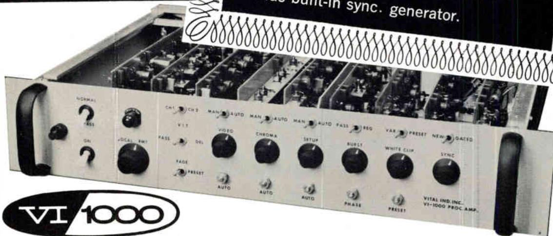
In one 3½" package, "Vital" Model VI-1000 video processing amplifier performs all these functions: VTR proc. amp.; stab. amp.; AGC, APC amplifiers; clamp amplifier; sync generator; color lock; video and burst distribution amplifiers; and all the automatic safeguards against FCC violations.
