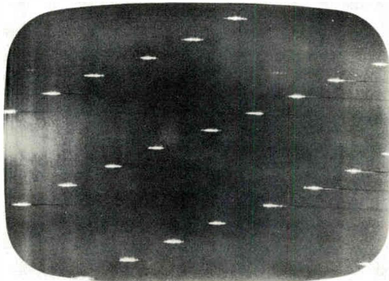
Any sharp object on the tape guides or heads can scratch the tape. This sharp object can be dirt, oxide debris, or a permanent burr.
