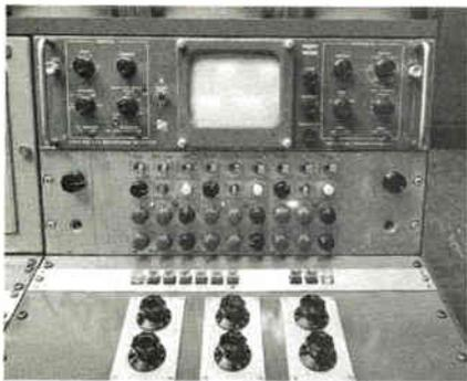
Fig. 8. The main operating controls on the remote camera-control console.
