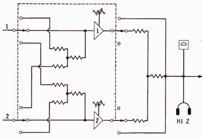
Fig. 2. Simpler version provides two microphone inputs.
