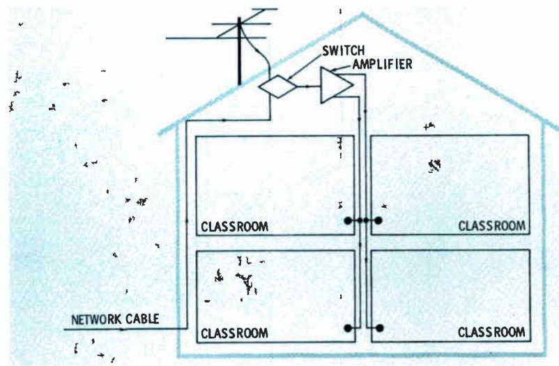
Fig. 6. Each school has been provided with cable and antenna signal sources.
