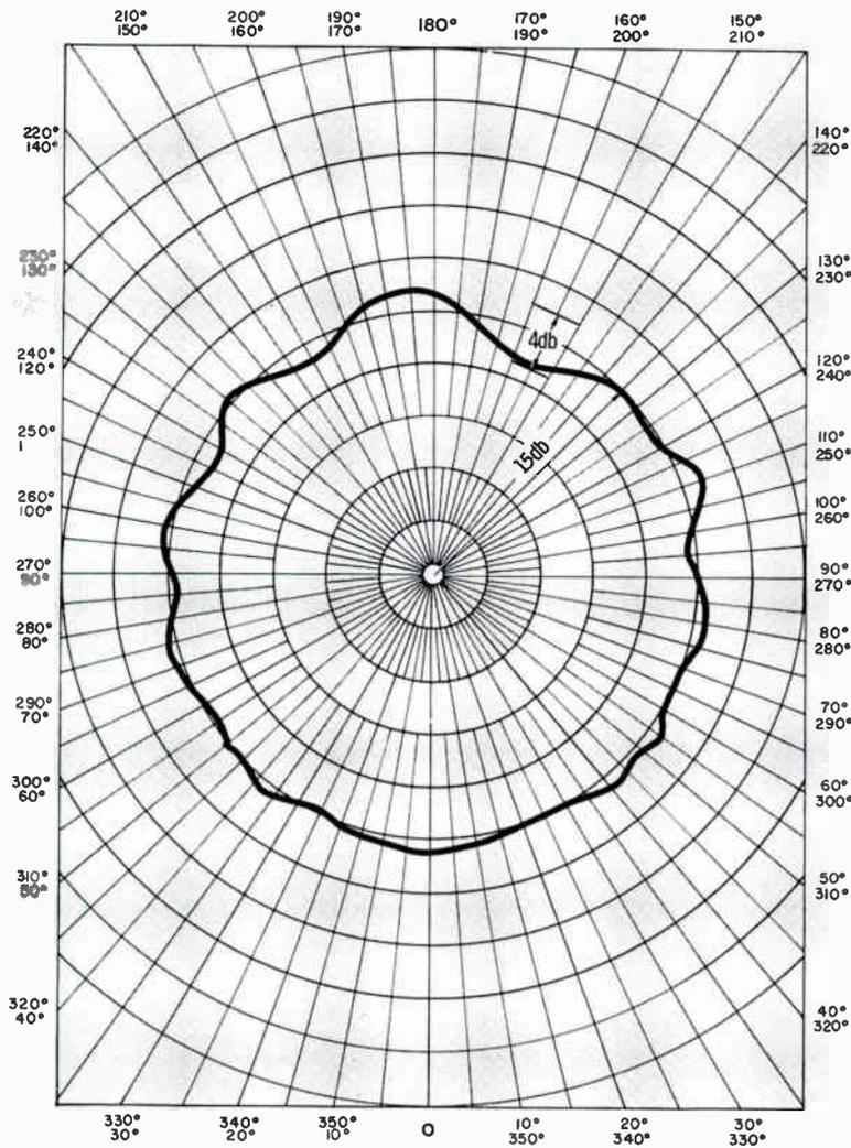
Fig. 3. Omnidirectional antenna pattern shows signal-strength nonuniformity.
