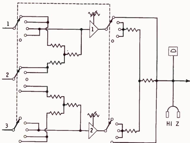
Fig. 1. Microphone No. 2 can be switched to both channels.
