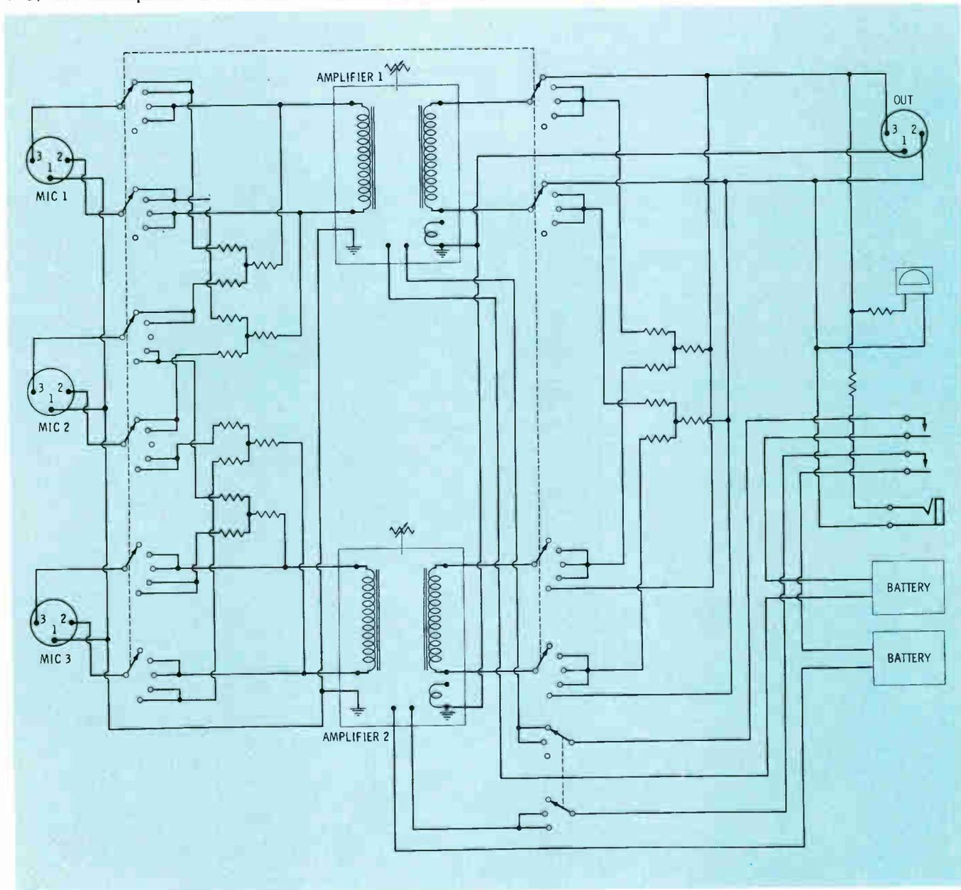
Fig. 3. Complete circuit of balanced redundant amplifier provides sophisticated operation with one ten-gang switch.
