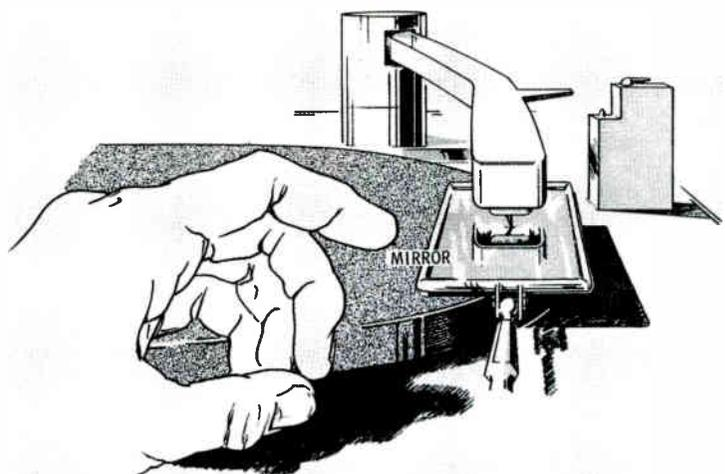
Fig. 2. Lateral tilt is easily measured with a mirror used to double angle.
