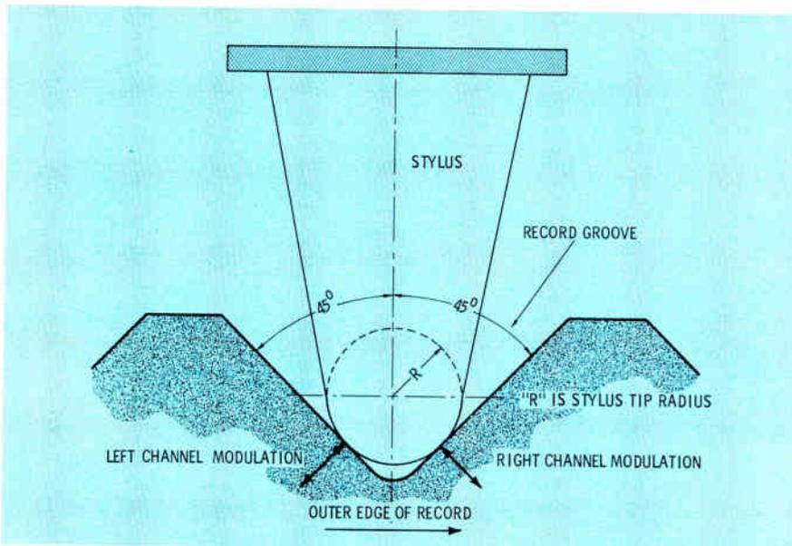
Fig. 4. Geometry of stereo record groove shows how stereo effect is achieved.
