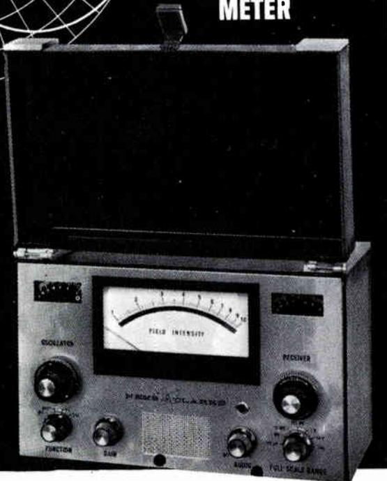
The new Model FIM-135 Field Intensity Meter provides exceptional reliability in the field due to its extremely ruggedized construction, solid-state design, and long life Mercury battery. Its lightweight (9 lbs.), compact (6½" x 10" x 6½"), and simplified design provides ease of handling and operation in the field.
