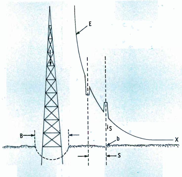
Fig. 2. The potential at the surface of the earth near an electrode containing lightning current. Note that the potential decreases as the distance from the tower is increased.
