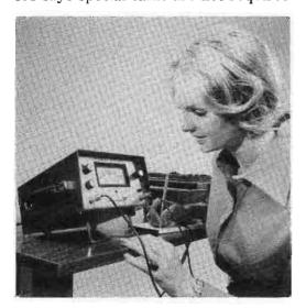
to operate the Model 6500. The instrument's "quick look" meter has calibrated color bands to indicate acceptable, marginal or unacceptable performance of the device being tested.
