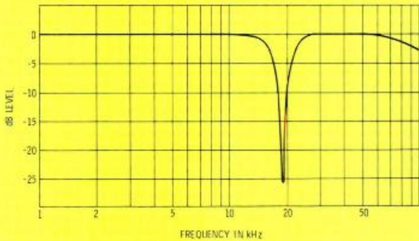
Fig. 1 Frequency response of a 19 kHz notch circuit.
