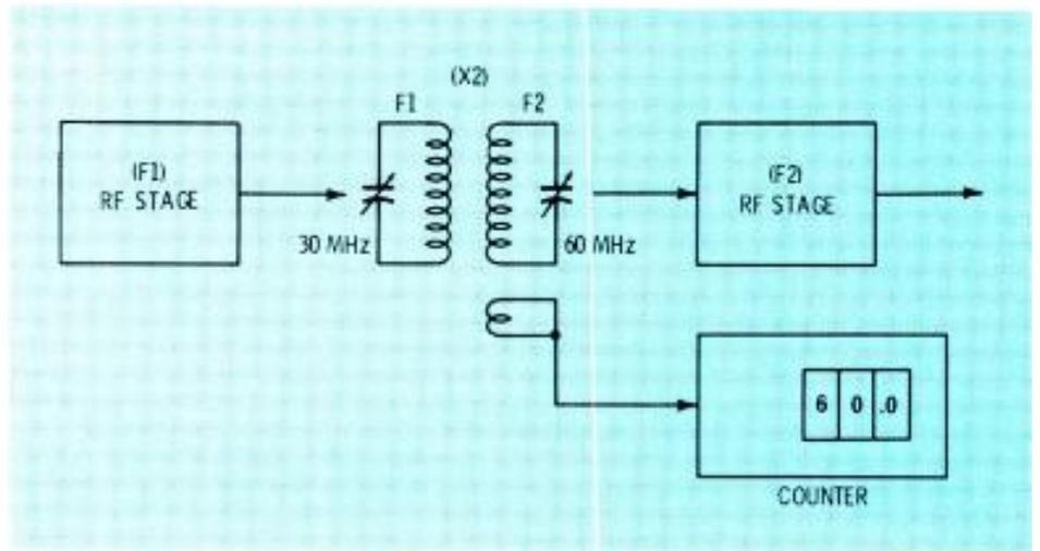
Fig. 4 Use tight coupling to the secondary of the RF transformer in a multiplier circuit.
