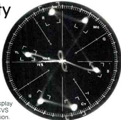
Typical Vectorscope display of VTR playback after CVS 504B time base correction.
