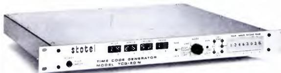
compatible with all other SMPTE code equipment and options plug in with no special tests or tools required. Our reader reads 80 bit SMPTE code from any source at speeds from hand turn to 40X. Self-contained character generator gives precise, single frame accuracy.
