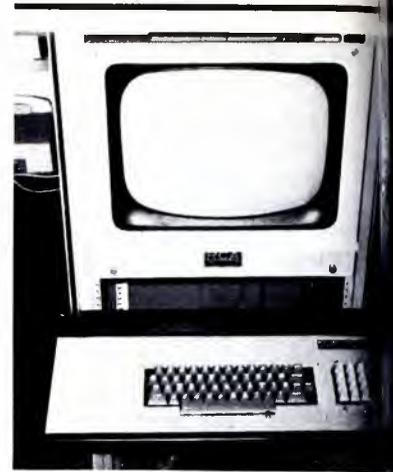
**Figure 2** This is an operator's eye of the keyboard and CRT. The board layout includes an auxiliary numeric pad on the right with controls cursor positioning and scrolling through the computer memory. This feature allows the operator directly examine and edit the menu contents. The Dataphone on the left is used to tie the system into Market for access to ARB data. The CRT is used by the operator at all times except when finished hardcopy is produced.
