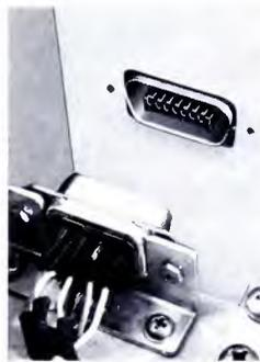
All leads to the deck go through this plug-in connector. There is nothing to disconnect to remove the deck.
