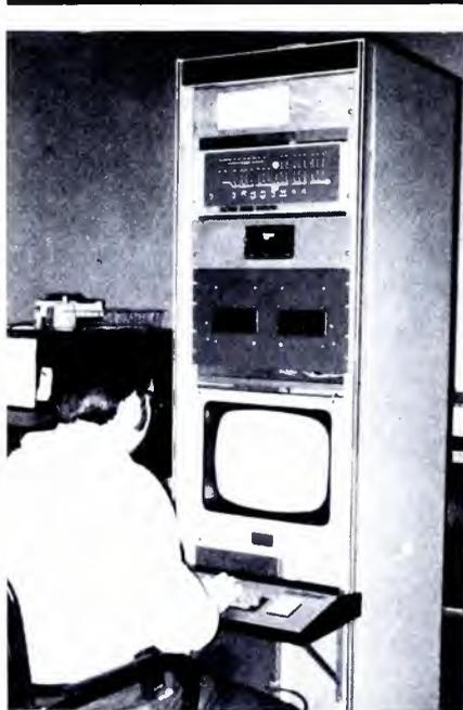
**Figure 1** The author is shown at the operating position of the computer system. From top to bottom the equipment is as follows: switching panel, Altair 8800 computer, mini floppy disc drive, digital cassette drives, video monitor, and keyboard. The system power supply (not in photo) is in the bottom of the rack.
