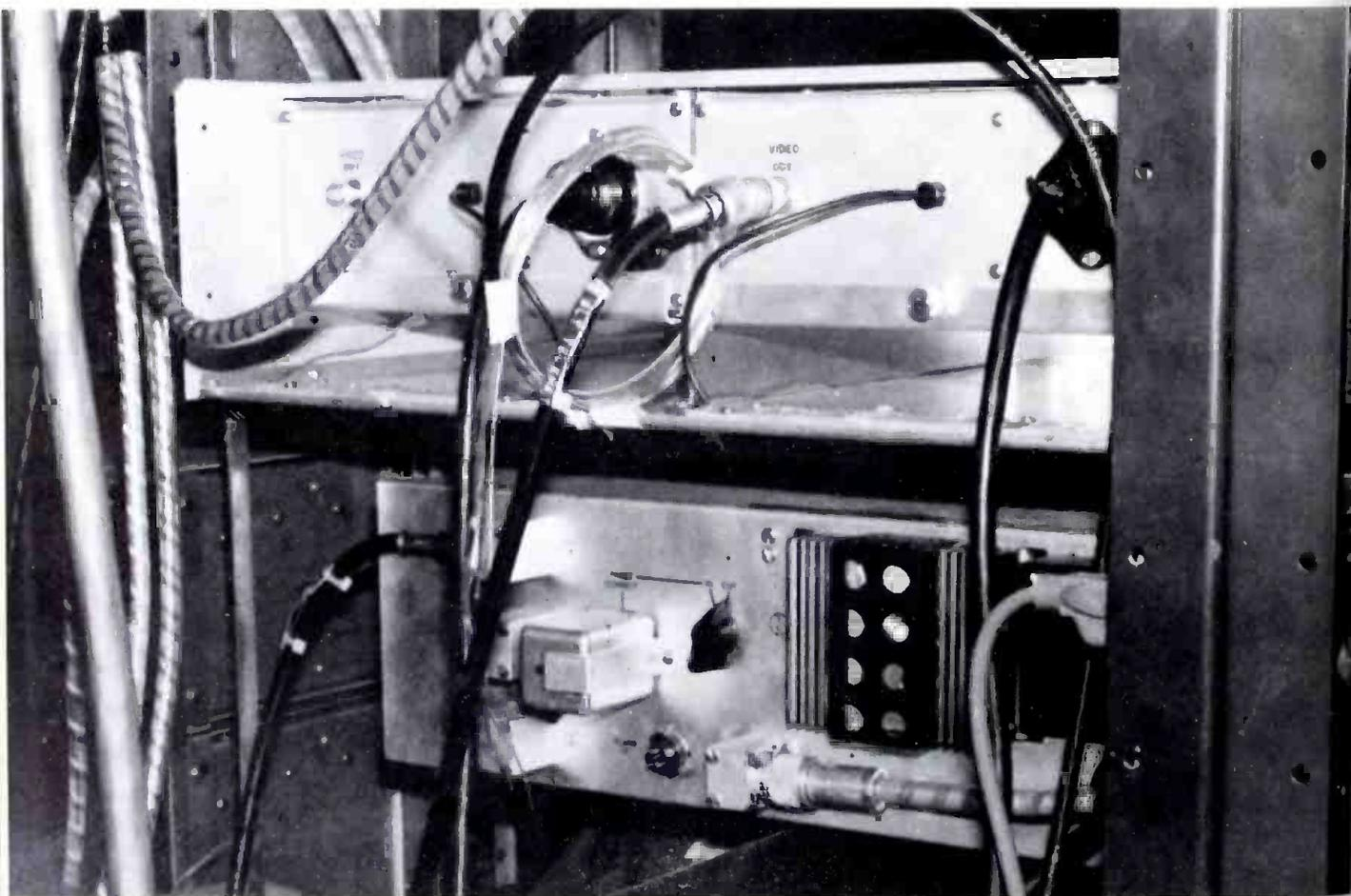
upper left photo shows the optic receiver mounted above the metallic cable receiver. The optic receiver was shown at the convention by Telemet. The lower left photo shows the back side of the rack with pigtailed to cable splices. They are taped to the back edge of the chassis. (Photos courtesy of KSL-TV)
