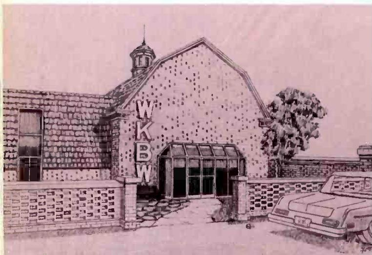
**Figure 1** New studios for WKBW, Buffalo, are being constructed in this turn-of-the-century carriage house. The addition on the left and the entire inside of the structure are totally new construction, with the flavor of wood and old brick retained to tie the building together with its surroundings in an historically significant neighborhood.
