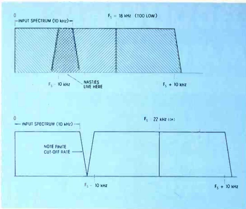
Figure 2 Upper diagram shows what happens if sampling rate is too low.
