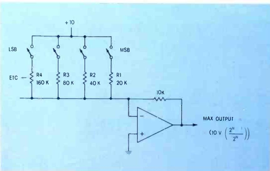
Figure 4 Simple D/A uses binary-weighted resistors.
