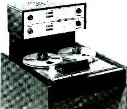
The AGC is designed for recording studios, radio stations and professional recording uses in the broadcast industry, education, industry and government. The 440C transport eliminates the problem of switching from fast forward-rewind to play by adding motion sensing. Edit control releases brakes, eliminating handling of the tension arm. Sapphire guides and a flutter idler reduce skew, thereby improving tracking.
