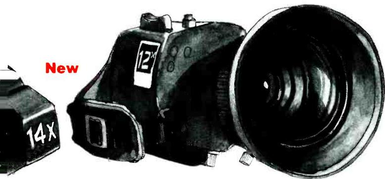
You'll see two new very lightweight zoom lenses for 1/2" format cameras. There's a 12x7 (7mm to 84mm) and 14x7 with built-in 2X extender (7mm to 196mm). Each offers F/1.4 speed, auto/manual iris, servo/manual zoom and focus. MOD is 0.8mm, weight 1.3kg.
