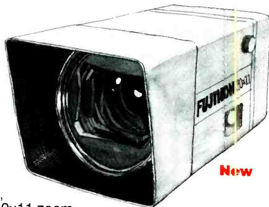
For field events, Fujinon's new 30x11 zoom with built-in 2X extender gives new range and flexibility to 2/3" format cameras. At maximum focal length of 660mm, it's the equivalent of 1,000mm on 1 1/4" format. Its F/1.6 aperture stays flat out to a 20X zoom. And at 30X, it gives you F/2.4. There isn't anything else in production that even comes close.
