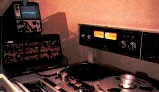
This view shows one of the KBIA Studer Revox B67 audiotape recorders. In the background is an Amber 4400A audio test set with a Tektronix T922 oscilloscope. As shown here, this setup is being used to check and align the frequency response of the recorder to assure optimum audio performance. The Amber test set can perform the roles of a function generator, tone burst generator, digital level and frequency meter, and spectrum analyzer.
