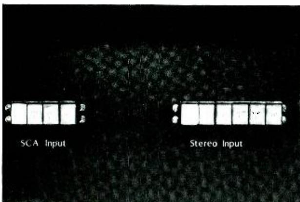
**KBIA broadcasts** a main channel and uses an SCA transmission as well. The passive switches shown here are used instead of patch panels to determine what goes into the main channel and what goes into the SCA.
