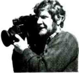
Compact new Color TV Camera carries off its broadcast standards oh, so lightly. One of the world's smallest, lightest ENG/EFP cameras. Ultra-light (only 9.7 lbs.) with shock-mounted optical system to deliver excellent picture quality, even under field conditions. 57 dB S/N ratio. 600-line resolution, auto digital white and black balance, true ABO, 2 ft. cand. intensity. Call Justina or Barbara for low daily/weekly rental rates.
