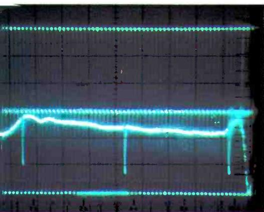
This is a close-up view of the oscilloscope screen as seen in the background above. This measurement shows a swept sine wave amplitude frequency response of the recorder. Shown here with the low frequency level being brought into alignment, the scope trace will be flat when alignment is achieved.
