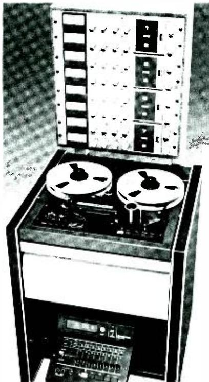
The MX-7800 is a 1-inch 8-channel recorder featuring 30/15ips; 600Ω balanced output; dc capstan-servo system; console cabinet; automatic monitor switching; VU meters plus peak LEDs; constant tape tension with dynamic braking; dual-frequency test oscillator; lift-up access to transport; and punch-in/punch-out.
