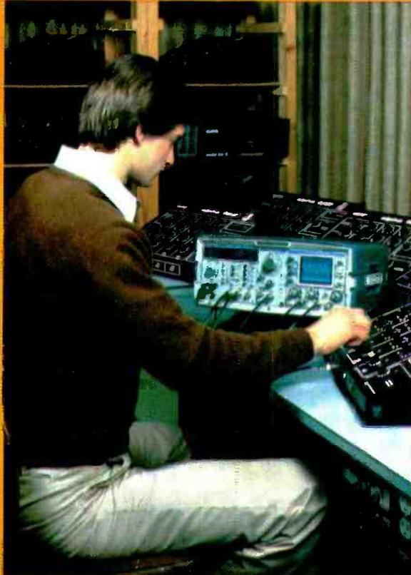
In addition to level and harmonic distortion measurements, the AA 501 measures intermodulation distortion to three standards: SMPTE, DIN and CCIF difference tone. Automatically selected.
