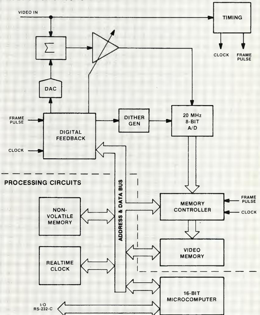
**Block Diagram.** The 1980 consists of two major circuitry blocks: acquisition and processing.
