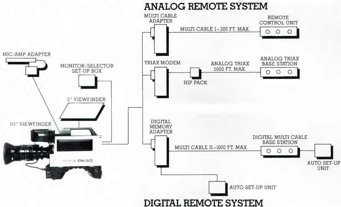
Introducing Toshiba's PK-60 ENG/EFP Color Camera. These drawings tell the story of the camera's digital and analog modularity. It features a separate digital memory with an internal microprocessor, an automatic setup unit with an 8-bit microprocessor, a digital base station and triax/wireless transmission with base station. The monitors also detail the PK-60's very modest dimensions.
