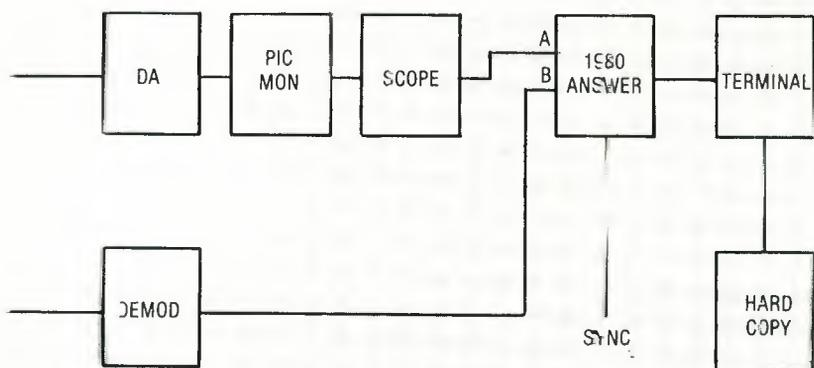
Figure 1 Typical 1980 ANSWER system test setup.
